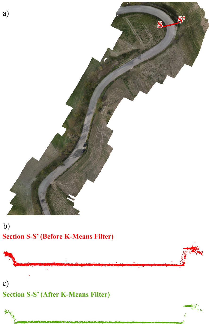
Figure 5.14 Road pavement section. a) Section S-S' (in red); b) Tie point cloud before the filter; c) Tie point cloud after the filter.
