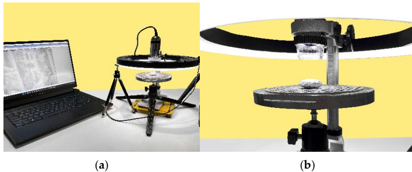
Figure 4. (a) Setup configuration for the first acquisition test, included calibrator, its support and lighting system; (b) Detail of the lighting ring coaxial to the rotating base, on which the calibrated plate is mounted.
