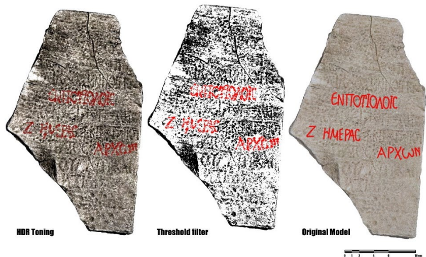
Figure 3. Lettering clearly distinguishable by DEM and RGB analysis overlaid on the orthoimage.
