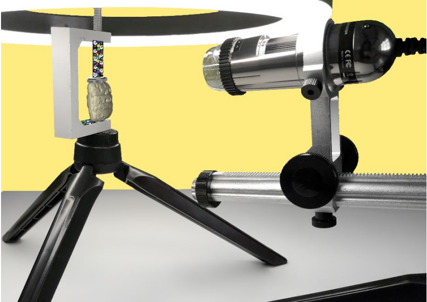
Figure 5. Three-dimensional calibrated plate combined with the digital microscope (updated prototype).
