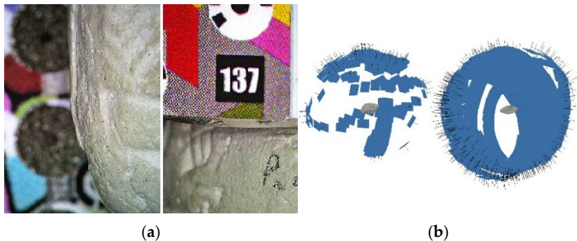
Figure 7. (a) Different ability to focus on target and object at the same time using the calibrated plate (left) or the clamp (right); (b) Camera spatial positions during the calibrated plate (left) and screw clamp acquisition test (same time taken: 1h).
