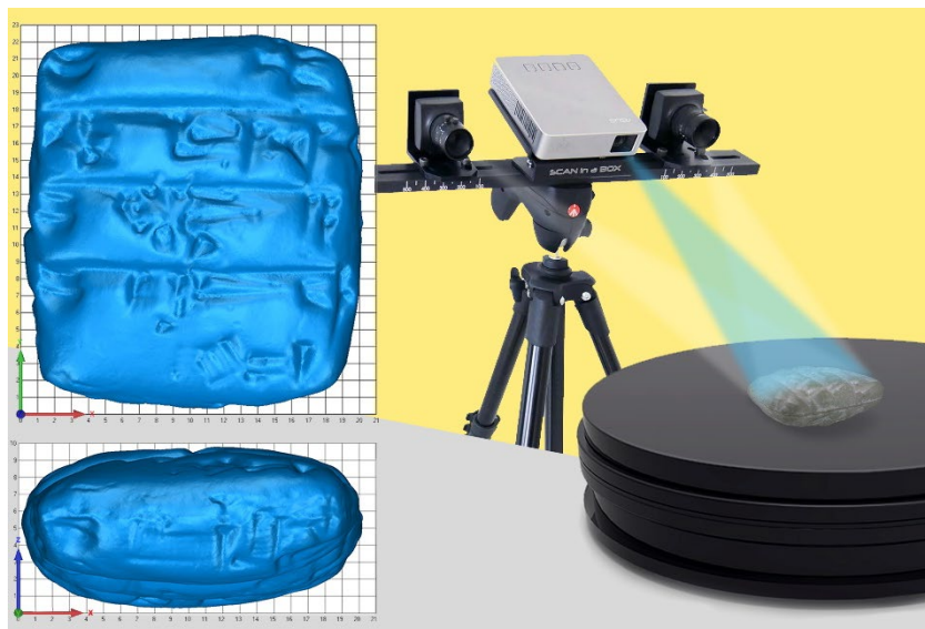
Figure 8. "SCAN in a BOX" system and polygonal model of the tablet acquired (1mm grid background).
