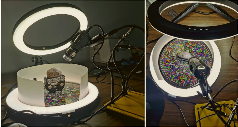
Figure 2. A turntable- and clamp-based acquisition system with ring illumination that supports integrated LED lighting of microscope. The USB microscope is fixed on a plastic micro-phone holder customized to be set to a plate with flexible hooks.
