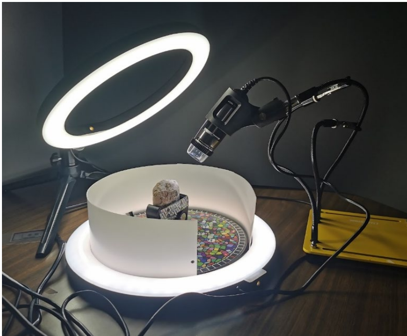
Figure 20. Acquisition system based on the turntable and clamp with ring illumination to support the microscope-integrated LED illumination. Magnification related to working distance: 20×.
