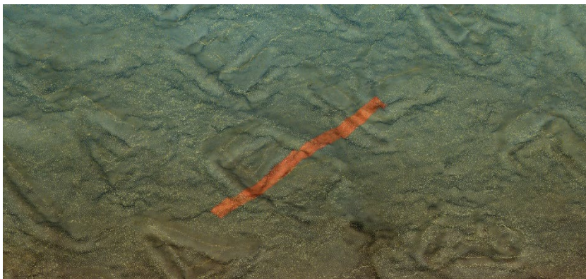
Figure 5. Photogrammetric cloud and resulting mesh (red one) generated by the 'micro system' (Dino-Lite).
