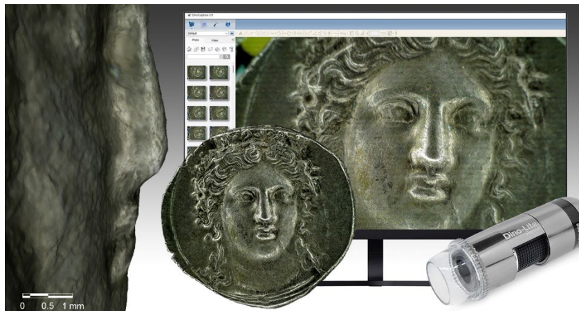
Figure 2. Zoom-in view and 3D model with texture mapping applied of the silver Croton strater acquired with Dino-Lite microscope.
