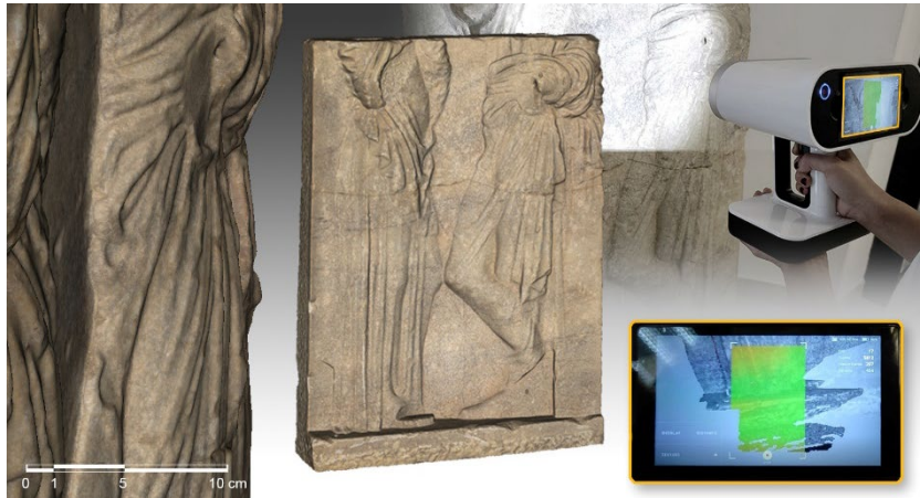
Figure 5. Zoom-in view and 3D model with texture mapping applied of the figurative relief acquired with Artec Leo scanner.
