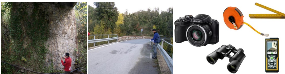
Figure 4.10 – Basic survey tools used for visual inspections [92]
