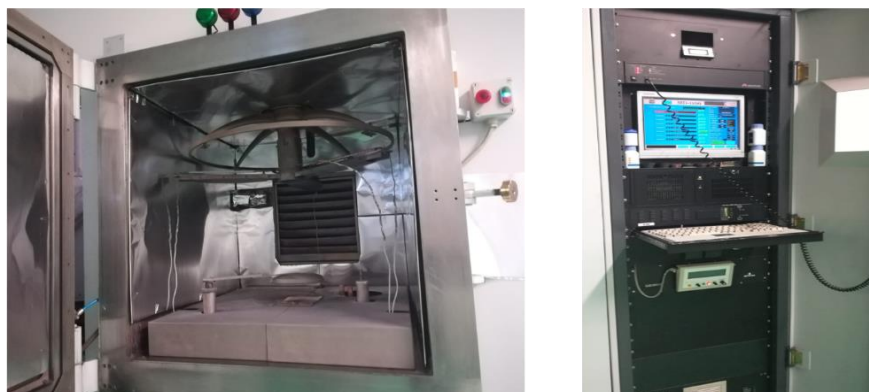
Figure D2: (a) electron-beam evaporator (b) thermal evaporator. Inside (right) and outside (left) of deposition systems. Adapted from [1].
