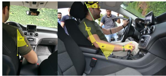
Figure 4-55: Angles acquisition during control knob use
