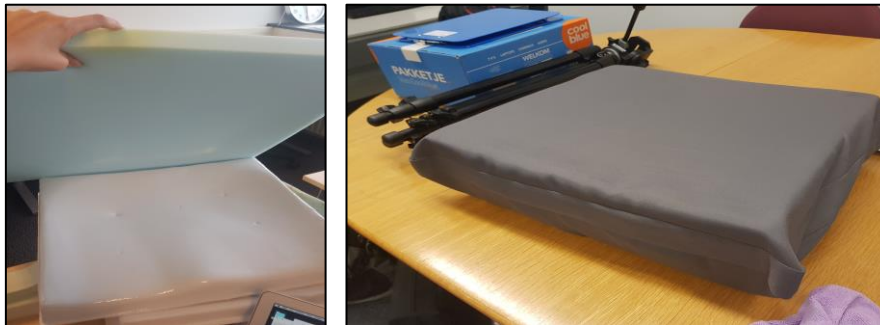
Figure 5-9: On the left: the prototype after thermoforming machine (to add the plastic layer) and the foam layer. On the right: the final model where the shape is hidden not to influence participants' expectations
