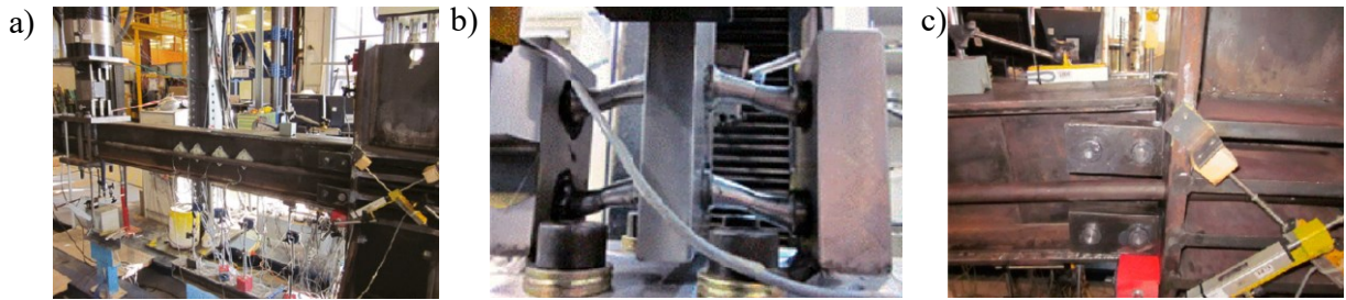
Figure 2.57. Vasdravellis et al. , 2012 [123] self-centring BCJ with WHPs: a) Overview of the specimen SC-WHP1; b) Detail of the WHP; c) Gap opening at 6% drift of specimen SC-WHP1
