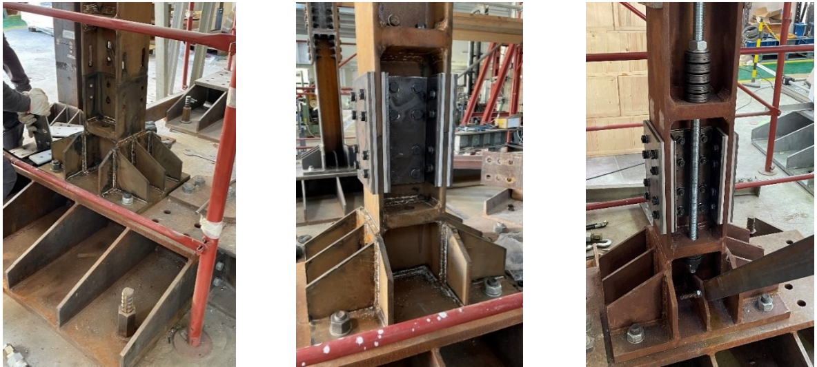
Figure 6.6. Assembly phases of the SC-CB connections
