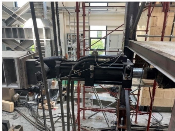
Figure 6.37. Actuator at the first storey.
