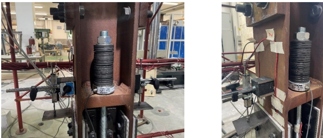
Figure 6.48. Details of the instrumentation for the FREEDAM BCJ
