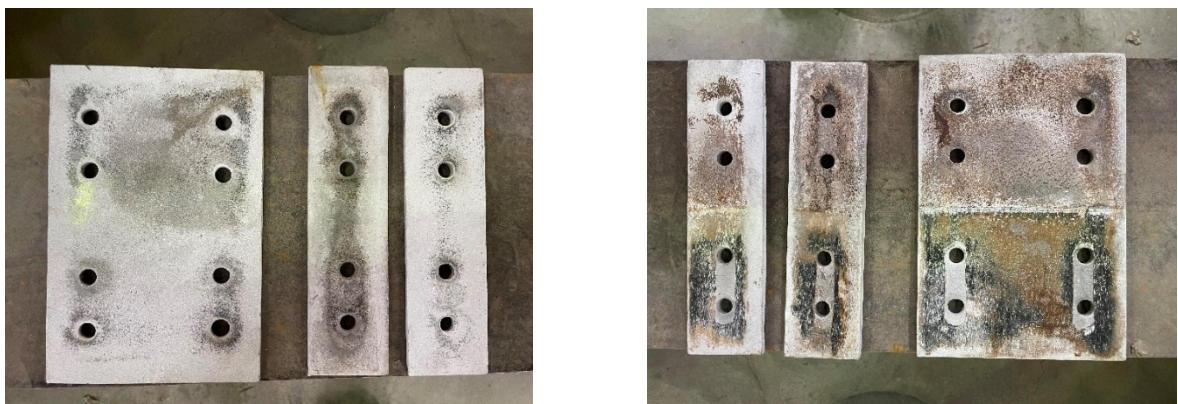
Figure 6.64. Test observations. Damage in the friction pads of the SC-CBs at the end of the experimental campaign
