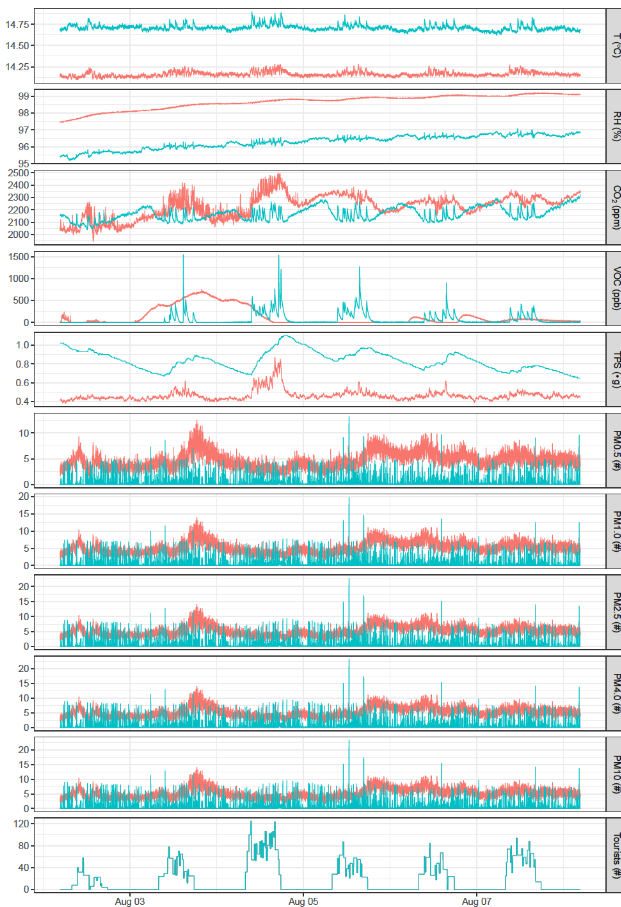
Fig. S2: Extract from the time series of all the parameters monitored (temperature: T, relative humidity: RH, CO 2 , VOC, typical particulate size: TPS, PM0.5, PM1.0, PM2.5, PM4.0, PM10) and of the number of tourists during the first week of August 2019 (from 2019-08-02 04:41:00 to 2019-08-08 04:41:00) in the tourist (green) and fossil (red) trails.
