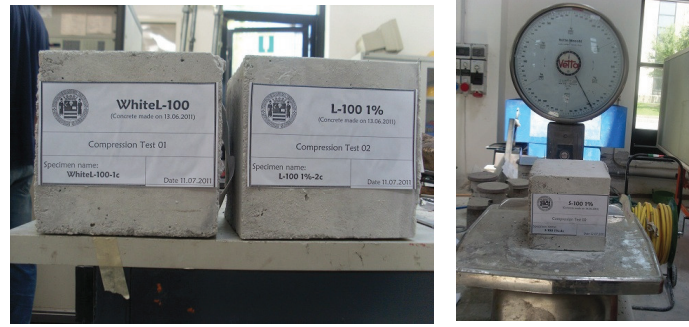
Figure 2.7: SFRC samples to be tested in compression.
