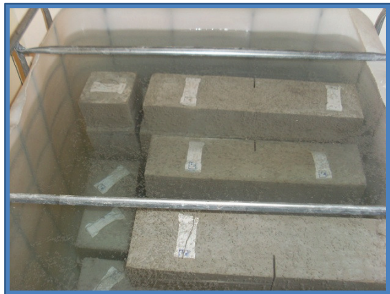
Figure 2.6: Underwater curing of specimens during 28 days at constant temperature of approximately 22°C.
