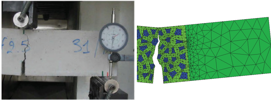
Figure 6.14: Crack paths of plain concrete and SFRC under three-point bending with central notch by Carpinteri and Brighenti [2010] .
