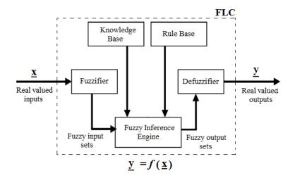
Figure 5.4: The general structure of a fuzzy logic controller
