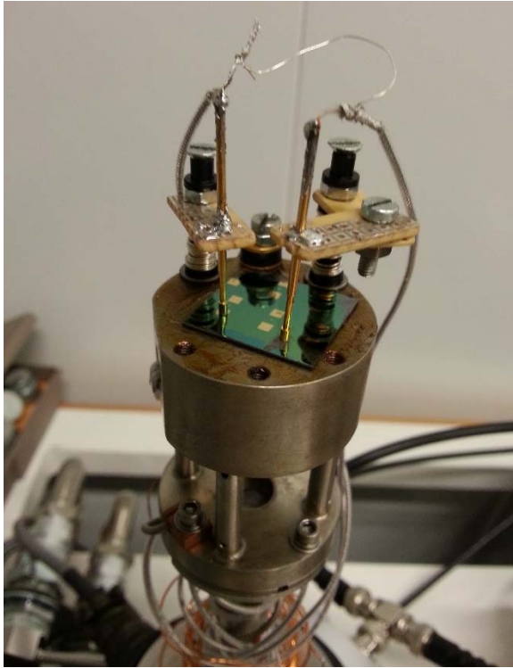
Figure 5.19. Devices were located in a cryostat for admittance measurements at different temperatures.
