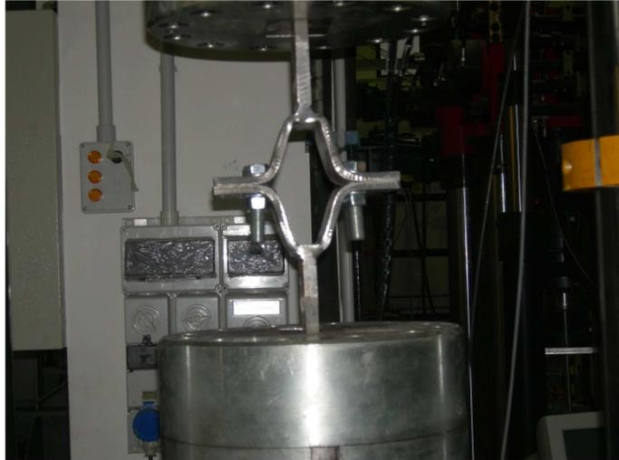
**Fig. 5.51** – Typical failure of TSD specimens
