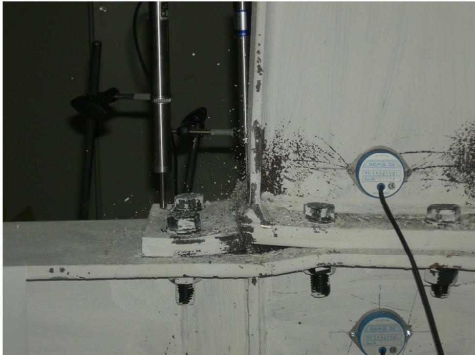
**Fig. 3.37** – Failure of the end-plate
