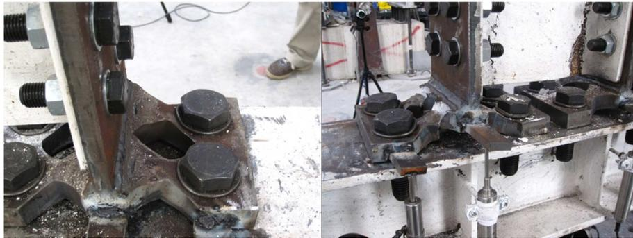
**Fig. 5.85** –Crack Formation and propagation (TSJ-XS-CYC 07)
