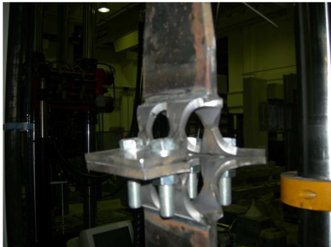
**Fig. 5.52** – Typical failure of TSD-XS specimens
