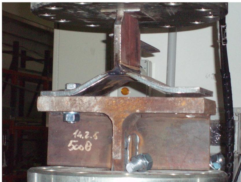
Fig. 5.43 – Typical failure of rectangular T-stubs on rigid support under monotonic loads
