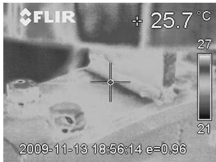
Fig. 5.56 – Propagation of the heat along the flanges – Rectangular T-stub
