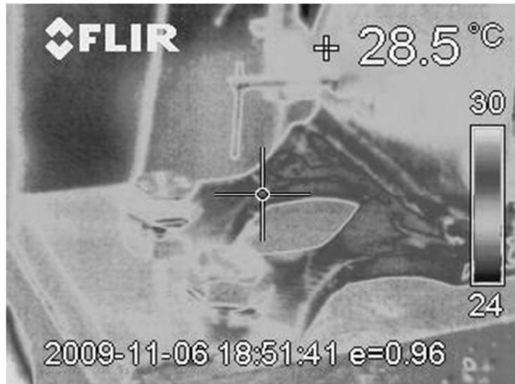
Fig. 5.55 – Propagation of the heat along the flanges – Hourglass T-stub
