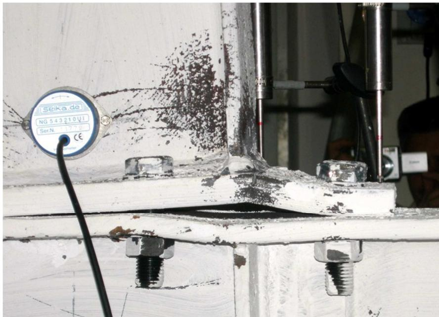
**Fig. 3.36** – Formation of the crack in the end-plate
