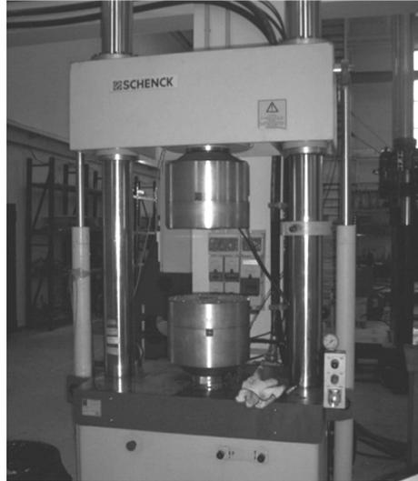
**Fig. 3.3** – Universal testing machine SCHENCK Hydropuls S56
