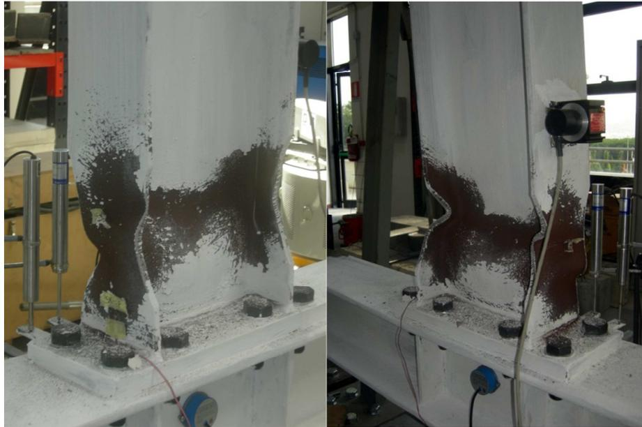
**Fig. 3.43** – Flange and web buckling
