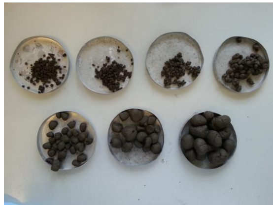
Figure 4.11 Examples of pellets at different process parameters
