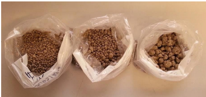
Figure 5.3 Aggregate produced from SW residues and PA
