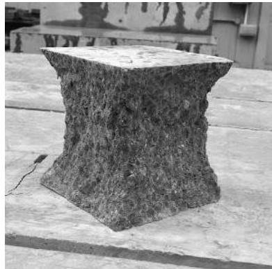
Figure 5.13 Concrete test cube with the failure mode due to compression
