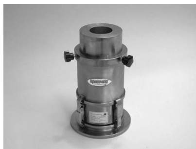
Figure 4.27 Steel cylinder for crushing resistance
