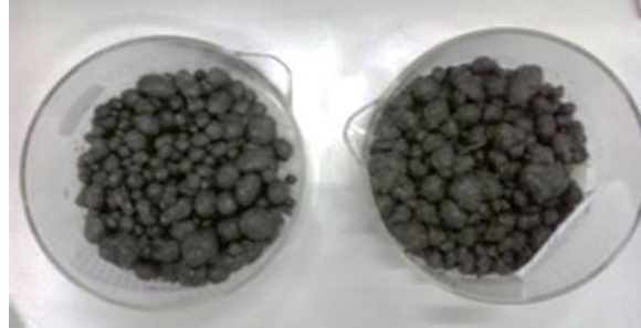
Figure 4.6 Granular materials obtained mixing artificial contaminated soil and cement.
