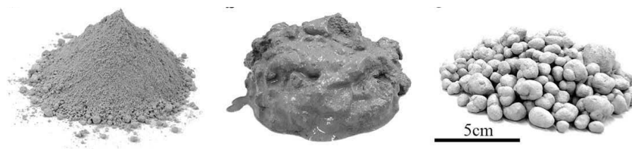
Figure 3.5 Example of a pelletised product developed by Gunning et al. (2009). These recycled materials have been tested to be used in lightweight concrete construction blocks (Figure 3.6).
