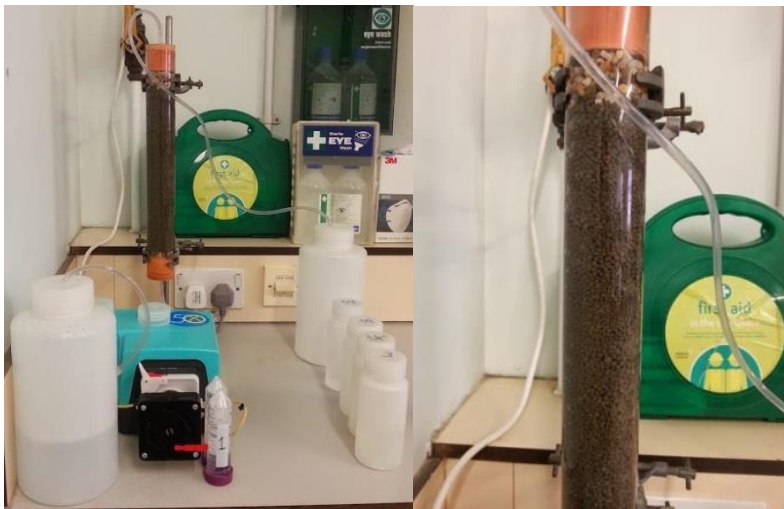
Figure 4.28 Apparatus set up for upflow percolation leaching test (prEN 14405)
