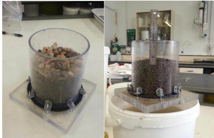
Figure 4.26 Cylindrical test sample for water permeability and maximum water capacity
