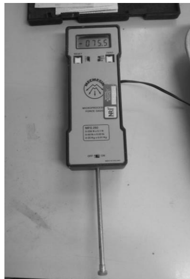
Figure 4.23 Hand-held force meter (Mecmesin MFG250)
