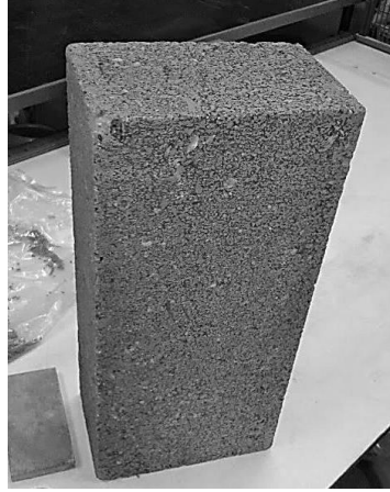
Figure 3.6 Example of block produced from recycled carbonated aggregate by Carbon 8 Aggregates Ltd (Gunning et al., 2012a).
