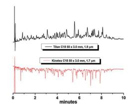
**Figure 4.13.** Comparison of a fast gradient elution on the Kinetex<sup>TM</sup> C18 50 × 3.0 mm. 1.7  $\mu$ m (red dotted line), Titan<sup>TM</sup> C18 50 × 3.0 mm, 1.9  $\mu$ m (black line). Instrument: Waters UPLC; Detector: PDA; Cell: 500 nL; UV at 214 nm; Tcol: 40 °C; Vinj: 6.0  $\mu$ L; Mobile phase: (A) H<sub>2</sub>O/ACN 95/5 v/v + 0.1% v/v TFA; (B) ACN/H<sub>2</sub>O 95/5 v/v + 0.1% v/v TFA; Flow rate: 1.5 mL/min. Sample: peptides < 3,000 Da fraction.
