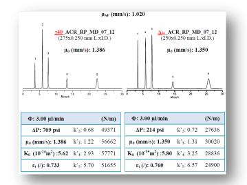
**Figure 1.9.** Comparison between monolithic columns obtained by radiation (left) and thermally (right) polymerization. 1: Uracil; 2: Benzaldehyde; 3: Nitrobenzene; 4: Ethylbenzene; 5: Butylbenzene.
