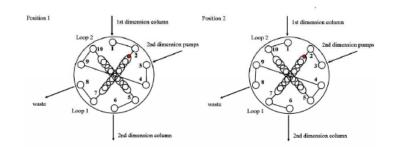
Figure 1.15. 10-port two-position switching valve.
