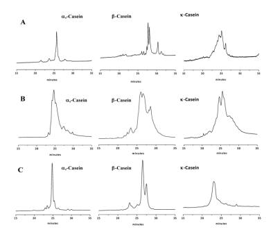
**Figure 3.2.** Chromatograms of casein standards on (A) a 27-cm long Protein-Cap-RP-Lauryl- $\gamma$ -Monolithic column (270 mm × 0.250 mm, L. × I.D.); (B) on an ACE C4 column packed with 3 µm particles (150 mm × 0.300 mm, L. × I.D.); and (C) on a Jupiter C4 column packed with 5 µm particles (150 mm × 0.300 mm, L. × I.D.). Gradient time: 30 min. Commercially available casein standards were dissolved in water. UV detection at 214 nm. See Section 3.2.4.1 for full experimental details.
