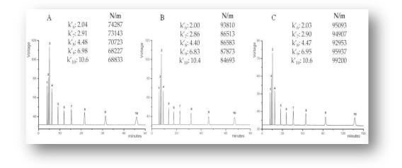
**Figure 4.2.** Chromatographic characterization and efficiency test of Protein-Cap-RP-Lauryl- $\gamma$ -Monolithic column (250 × 0.250 mm L. × I.D.). (A):  $\Phi$ : 3.00  $\mu$ L/min,  $\Delta P_c$ : 817 psi; (B)  $\Phi$ : 2.00  $\mu$ L/min,  $\Delta P_c$ : 523 psi;  $\Phi$ : 1.00  $\mu$ L/min,  $\Delta P_c$ : 287 psi.
