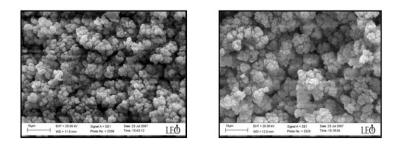
**Figure 1.8.** Comparison between monolithic polimer obtained by radiation (left) and thermally (right) polymerization.
