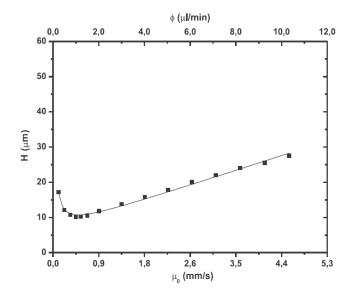
**Figure 4.3.** Experimental van Deemter for n-pentyl-benzene, column: Protein-Cap-RP-Lauryl- $\gamma$ -Monolithic column (250 × 0.250 mm, L. × I.D.). Mobile phase: ACN/H<sub>2</sub>O; 60/40,  $\nu/\nu$ ;  $\eta$ : 0.72 × 10<sup>-3</sup> Pa s at 25 °C. Column oven: 25 °C; Detection: UV at 214 nm. Injection volume: 50  $\eta$ L.
