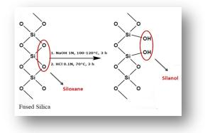
Figure 1.4. Activation of inner wall surface of fused silica capillary.
