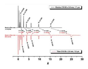
**Figure 4.12.** Comparison of isocratic elution on the Kinetex<sup>TM</sup> C18 50 × 3.0 mm, 1.7  $\mu$ m (black line), Titan<sup>TM</sup> C18 50 × 3.0 mm, 1.9  $\mu$ m (red dotted line). Column oven: 35 °C; Detection: UV at 214 nm, Sampling rate: 80 points/s; resolution: 4.8 nm; no filter. Injection volume: 0.5  $\mu$ L. Sample: small molecule mixture. Results are expressed as retention factors (k) and theoretical plates per column (N).
