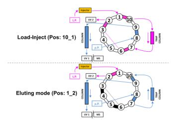
Figure 3.1. Sketch of 10-valve port used for load-trapping purposes.
