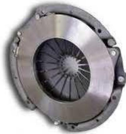
**Figure 2.20:** Pressure plate
