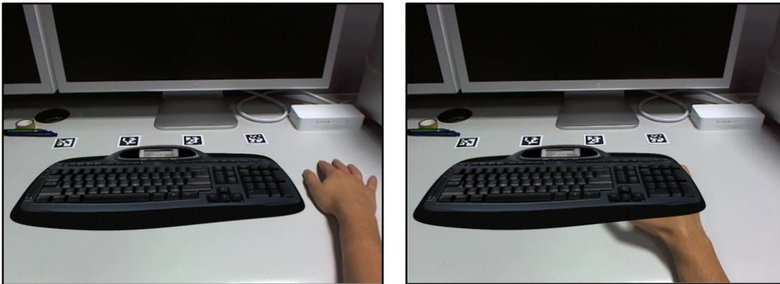
**Figure 12.** *Left: A virtual model of a keyboard rendered onto a captured frame of real environment to augment it. The hand positioned along the right side of the keyboard does not ruin the Mixed Reality illusion. Right: The same MR scene, but as the hand is positioned over the keyboard, it is occluded by the virtual content.*
