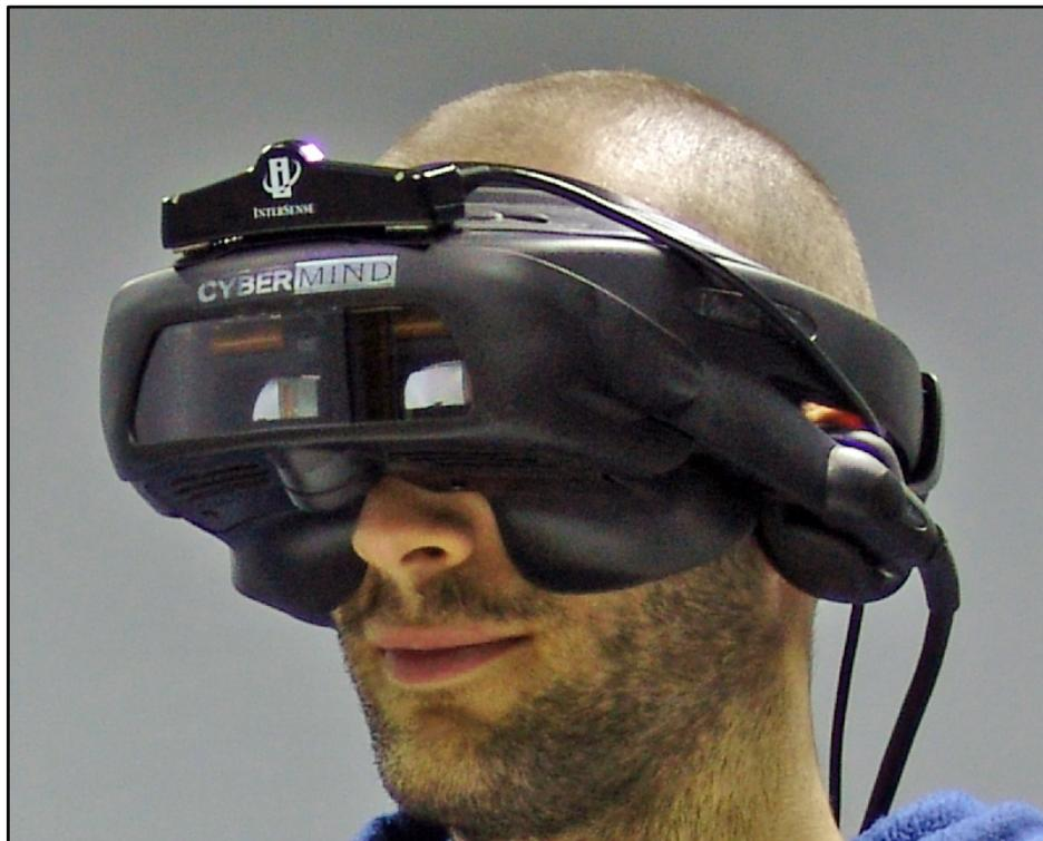
**Figure 5.** *A close up view of the Cybermind optical see-through HMD worn to visualize the virtual contents onto the real environment.*
