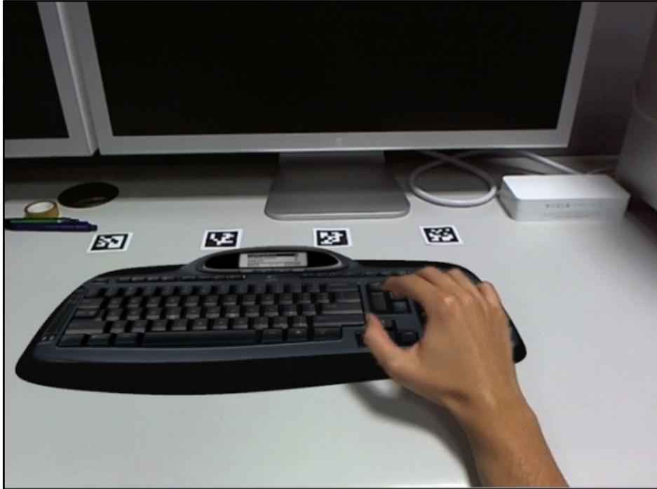
**Fig. 16.** *Compositing and final result. The original real background shown in Fig. is composited according to the disparity map of the scene enabling a correct visualization and a meaningful interaction (note that hand's casted shadow is not currently handled by the proposed method).*
