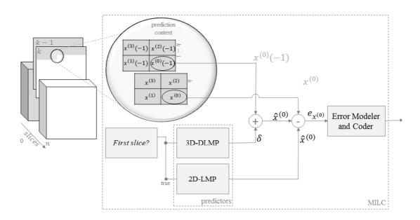
Figure 3.1: The MILC diagram block (adapted from [20]).
