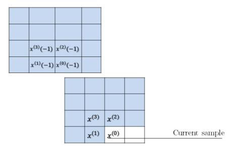
Figure 3.3: A graphical example of the prediction context used by the 3D-DLMP predictor.
