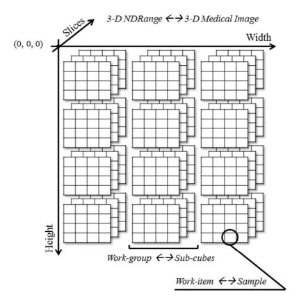
Figure 3.10: Graphical representation of the mapping of MI into work-groups (from [47]).
