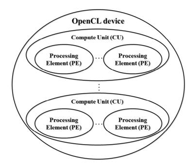
Figure 3.9: Graphical representation of the logical architecture of an OpenCL device.
