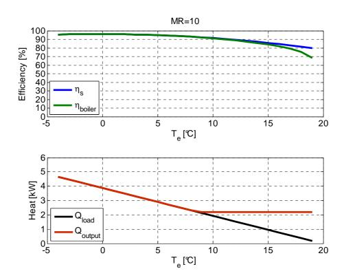
Figure 30. For a boiler with maximum modulation ratio equal to 10: in top figure the efficiency degradation due to cycling losses, in the second one, boiler heat output and loads as a fuction of external temperature.
