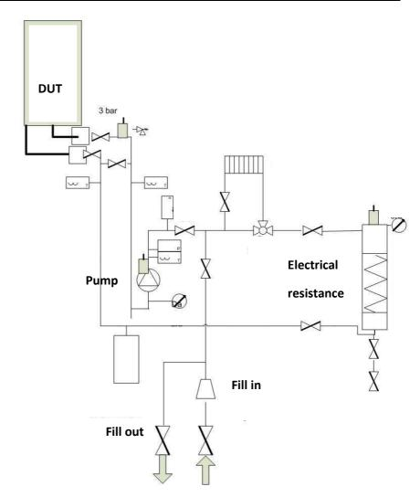
Figure 15. Insulation measurement test rig composed by electrical resistance and pump controlled by PID in order to deliver constant temperature water
