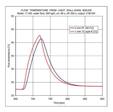
Figure 4. Transient measurement comparison between a 1mm thermocouple and a 3mm thermoresistance
