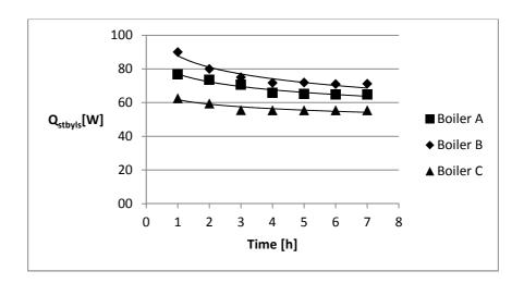
Figure 17. Boiler standby losses results for three differently insulated boilers
