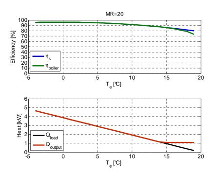
Figure 31. For a boiler with maximum modulation ratio equal to 20: in top figure the efficiency degradation due to cycling losses, in the second one, boiler heat output and loads as a fuction of external temperature
