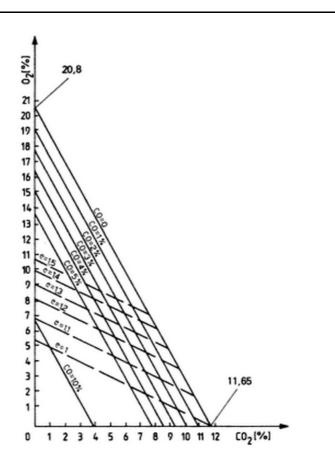
Figure 23. Ostwald triangle for methane – The triangle correlate air excess "e" with CO, CO<sub>2</sub> and O<sub>2</sub> concentrations determining the combustion conditions.
