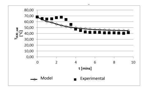
Figure 20. Experimental and model water temperature draw-off for a 22kW and 40liters storage boiler and a 10l/min flow rate. Experimental draw-off show firstly a peak due to tank temperature stratification and following a valley, whereas modeled temperature maintains an average value
