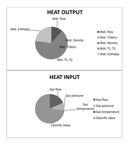
Figure 3. Relative weight of different measurements on the heat input and heat output uncertainty
