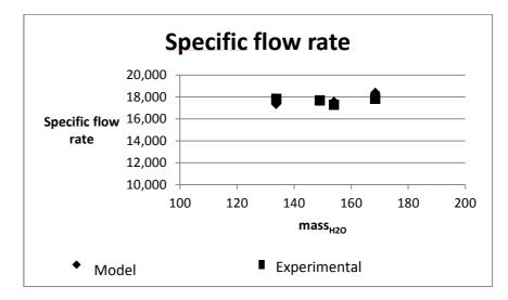
Figure 21. Experimental and modeled specific flow rate is reported for different tapped water quantities for a 22kW and 40 liters storage boiler. Model well approximates SR experimental results.
