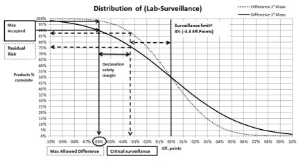
Figure 14. Surveillance tollerance on water efficiency analysis on storage water heater assuming an acceptable risk of non-conformity.
