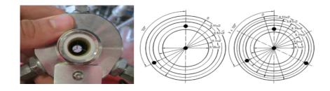
Figure 5. Thermocouples positioning with surface methods.
