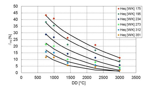
Figure 34. Model results and relation between degree days and total energy saving due to ultra-modulation for different building specific heat losses.
