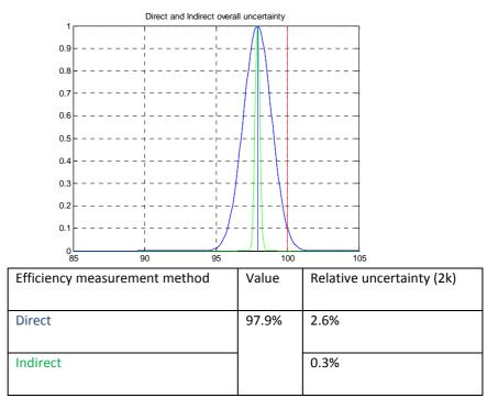
Figure 6. Comparison of direct and indirect estimation of efficiency in terms of measurement uncertainty
