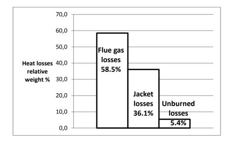
Figure 7. Relative weight of losses terms on the global heat loss of a boiler
