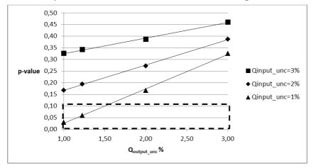
Figure 10. Measurement system design criteria based on statistical closure of energy balance.
