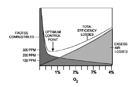
Figure 22. Boiler combustion loss as a function of oxygen concentration in the flue gas, which is correlated to the air excess.
