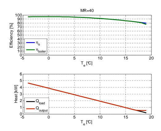
Figure 32. For a boiler with maximum modulation ratio equal to 40: in top figure the efficiency degradation due to cycling losses, in the second one, boiler heat output and loads as a fuction of external temperature.
