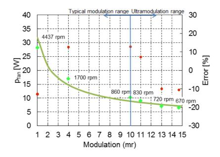
Figure 29. Experimental and modeled fan electrical consumption and relative error for different fan rpm and modulation ratio. Data is divided into modulation and ultra-modulation range.
