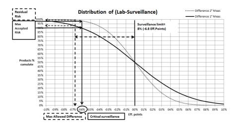
Figure 13. Surveillance tollerance on water efficiency analysis on storage boiler assuming an acceptable risk of non-conformity.
