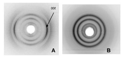
**Fig. 2.2.8** Photographic X-ray diffraction patterns of the same films of Fig.2.2.7C (A) edge, obtained with X-ray beam parallel to the film plane by using a cylindrical camera, recorded on a imaging plate and (B) trough perpendicular to the film plane.
