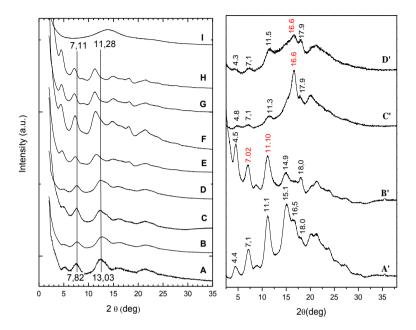
**Fig. 2.2.9** X-ray diffraction, collected by an automatic powder diffractometer, (A-I) trend of different nanoporous crystalline phase. (A) benzene; (B) tertralin; (C)  $CH_2Cl_2$ ; (D) DCE; (E)  $\alpha$  pinene; (F) TCB; (G) clorodecane; (H) CCl<sub>4</sub>; (I) decalin
