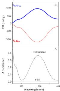
**Fig. 3.8**. UV–vis (A) and CD (B) spectra, in the range 275–400 nm, of s-PS 6  $\mu$ m films, exhibiting the  $\delta$  clathrate phase with NA, with NA content close to 1.7 wt %. Thin red line and thick blue line correspond to films first crystallized by sorption of (R)-(–) carvone or (S)-(+) carvone, respectively.
