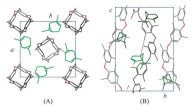
**Fig. 3** Packing model of the co-crystalline form of PPO with (1S)-(-)- $\alpha$ -pinene in the unit cell a= b = 1.19 nm and c = 1.71 nm, and the P4<sub>3</sub> space group (A) Projection along c; (B) projection along a. None bonded distances are all longer than 0.36 nm.
