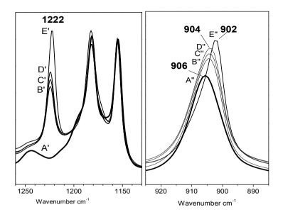
**Fig 2.4.5** FTIR transmission spectra in the wavenumber range 1130-1260 cm<sup>-1</sup> of amorphous s-PS film after annealing: (A'), mesomorphic transplanar (B'-D') obtained by annealing amorphous films at 130°C for 1h (B'),2h(C') 3h(D'), and crystalline  $\alpha$  form films (E') and 925-885 cm<sup>-1</sup> (A''-E'')
