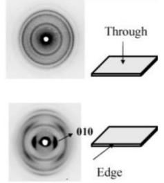
**Fig.2.4.2**. X-ray patterns taken with beams perpendicular (THROUGH) and parallel (EDGE) to the film plane on a photographic cylindrical camera of the  $\delta$  "uniplanar" oriented co-crystalline phase including DCM.
