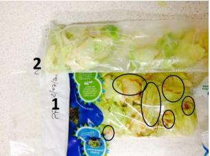
**Fig 2.4.12** Salad packaging in BOPP film and in PP-sPS-PP crystallized film. With symbol O maceration are indicated
