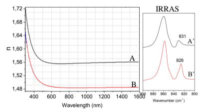
**Fig. 4.3.9** Refractive index n of PPO thin film versus wavelength: A) Amorphous PPO ( black line); B) PPO nanoporous crystalline structure by benzene (red line). The respective IRRAS spectra (A'-B') are reported.
