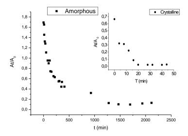
**Fig. 4.3.6** Desorption at room temperature, in amorphous (**■**)and crystalline (**●**) samples of PPO \CCl<sub>4</sub>. ( $A_t = 786 \text{ cm}^{-1}$ ) is a CCl<sub>4</sub> vibrational peak normalized respect to a PPO reference peak 960 cm<sup>-1</sup>( $A_o$ ).  $A_t/A_0$  are reported versus the desorption time.
