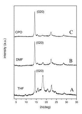
**Fig. 2.3.3.** X-ray diffraction, as collected by an automatic powder diffractometer of PLLA films presenting  $\epsilon$  PLLA co-crystalline phases with THF (A), DMF (B) and CPO (C) guest molecules.
