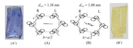
**Fig. 3. 1.** Packing of  $\delta$ -clathrates of s-PS with azulene (A, monoclinic) and NA (B, triclinic). Only a couple of enantiomorphous polymer helices (R = right-handed, L = left-handed) that confine the guest molecule are shown. The NA guest (B) is accommodated by the shifting the ac layers along the chain axis, leading to the triclinic symmetry. Blue (A') and yellow (B') s-
