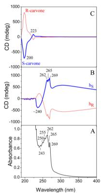
**Fig. 3.3** UV–vis (A) and CD (B) spectra of s-PS amorphous films, with a thickness of ~6  $\mu$ m, after (R)-(–) carvone (red thin line) or (S)-(+) carvone (blue thick line) induced crystallization. (C) CD spectra of s-PS spin-coated amorphous films, having a thickness of ~0.3  $\mu$ m, subjected to the same treatments.
