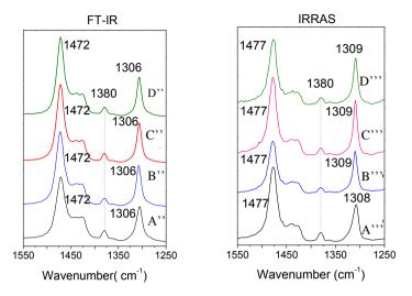
**Fig. 4.3.3** FT- IR (A-D) and IRRAS (A'-D') spectra in the 1225-1170 cm<sup>-1</sup> wavenumber range, FT- IR (A''-D'') and IRRAS (A'''-D''') spectra in the 1550-1250 cm<sup>-1</sup> wavenumber range. Trend of different nanoporous crystalline phase of PPO: (A) Amorphous; (B) 1,2-dichlorobenzene; (C) CCl<sub>4</sub>; (D) limonene.
