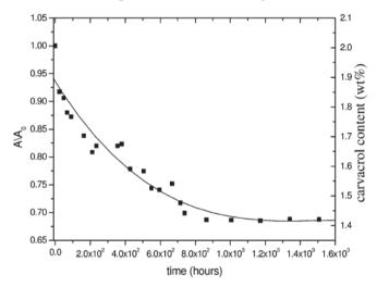
**Fig. 1.14** Carvacrol desorption at 35 °C from a s-PS film with a carvacrol content of 2.1 wt % with most molecules being guest of the s-PS crystalline phase.
