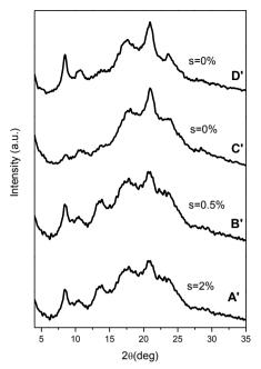
**Fig. 2.4.6** X ray diffraction patterns of mesomorphic trans-planar (A-C), as well as crystalline  $\alpha$  form films (D)after exposition to DCM vapors for 15-30 minutes respectively. Shrinkage values (s) are also reported.
