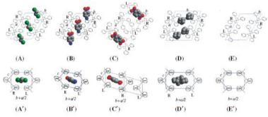
**Fig. 1.1** Schematic projections along the chain (up) and perpendicular to the chain (down) of s-PS co-crystalline forms: A, A' monoclinic  $\delta$ -clathrate form with 1,2-dichloroethane <sup>10</sup>, B, B' triclinic  $\delta$  -clathrate form with p-nitroaniline <sup>4</sup>, C, C' triclinic  $\delta$  -clathrate form with 1,4-dinitrobenzene <sup>5</sup> D, D' intercalate form with norbornadiene <sup>11</sup>, and E, E' monoclinic  $\delta$  -nanoporous phase <sup>12</sup>
