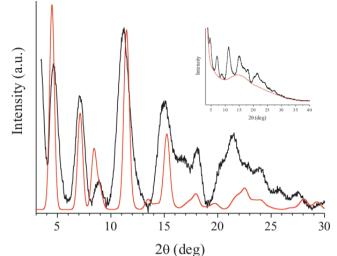
**Fig. 2.2.14** comparison between the calculated x-ray diffraction profile (red) according to the structural model of figure 1.15 vs. experimental X-ray diffraction pattern (black), after substraction of amorphous and backgroup contribution
