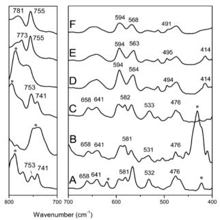
**Fig 2.2.6**. FTIR spectra in the 800–700 and 700–400 cm–1 ranges of unoriented PPO films: (A) cocrystalline with  $\alpha$ -pinene; (B) cocrystalline with tetralin; (C) cocrystalline with decalin; (D) cocrystalline with carbon
