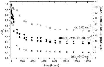
**Fig. 1.16** Reduced absorbance of carvacrol infrared bands of guest molecules only in the crystalline  $(3532 \text{ cm}^{-1})$  or only in the amorphous  $(3400 \text{ cm}^{-1})$  or in both phases (2960, 1420, and 809 cm<sup>-1</sup>), versus desorption time. On the right scale, the overall carvacrol content in the film, as determined by thermogravimetry
