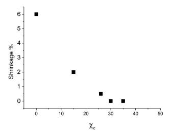
Fig 2.4.7 The % shrinkage after crystallization procedure versus crystallinity degree  $\chi_{cIR}$
