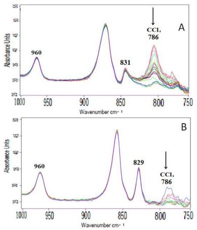
**Fig 4.3.5** FTIR transmission spectra in the wavenumber range 1000–750  $\text{cm}^{-1}$  of amorphous PPO/CCl<sub>4</sub> film (A) at 36h; and crystalline PPO/CCl<sub>4</sub> film (B) at 40 min.
