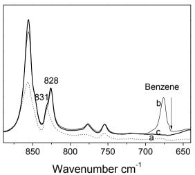
**Fig 4.2.4** FTIR transmission spectra in the wavenumber range 900-650 cm<sup>-1</sup> of PPO in PhC has collected (a) amorphous PPO (dot line); (b) co-PPO\benzene crystal (thin line); (c) extracted by  $CO_2$  (thick line)
