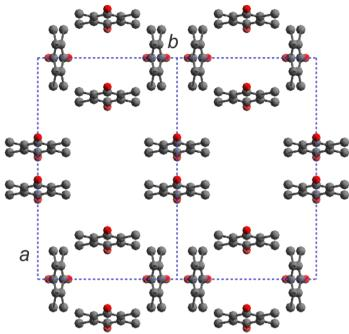
**Fig. 2.2.13** Packing model of the nanoporous PPO form in the unit cell a = 19.72 Å; b = 12.4 Å; c = 10.6Å;  $\alpha = \beta = \gamma = 90$  and P222<sub>1</sub> space group.Projection along c
