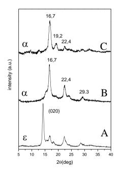
**Fig.2.3.10** X-ray diffraction patterns of PLLA film exhibiting (020) uniplanar orientation of the co-crystalline phase with DMF, before (A), after extraction with supercritical  $CO_2$  (B), after guest desorption at room temperature (C).
