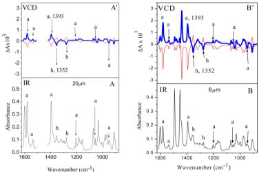
**Fig. 3.5.** FTIR (A, B) and VCD spectra (A', B') of s-PS films, having a thickness of nearly 20  $\mu$ m (A, A') or 6  $\mu$ m (B, B'), after crystallization induced by (R)-(–) carvone (thin red line) or (S)-(+) carvone (thick blue line) and exchange of the nonracemic carvone guest with the achiral azulene guest. The azulene content is close to 14 wt %. The main peaks of the azulene guest molecules are labeled by "a" while some typical polymer host peaks are indicated by "h".
