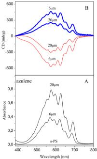
**Fig. 3.6.** Visible (A) and CD (B) spectra, in the range 400–800 nm, of s-PS films, with thickness of 20 and 6  $\mu$ m, after (R)-(–) carvone (red thin line) or (S)-(+) carvone (blue thick line) induced crystallization and replacement of the nonracemic carvone guests with the achiral azulene guest
