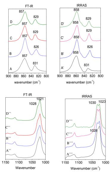
**Fig 4.3.2** FT- IR (A-D) and IRRAS (A'-D') spectra in the 900-800 cm<sup>-1</sup> wavenumber range, FT- IR (A''-D'') and IRRAS (A'''-D''') spectra in the 1150-1000 cm<sup>-1</sup> wavenumber range. Trend of different nanoporous crystalline phase of PPO: (A) Amorphous; (B) 1,2-dichlorobenzene; (C) CCl<sub>4</sub>; (D) limonene.
