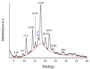
**Fig. 2.3.5.** X-ray powder diffraction pattern of an unoriented sample of PLLA-CPO clathrate form. The presence of a reflection centered at  $2\theta$ =16.7° points out the presence of a minor amount of residual PLLA in  $\alpha$  form. The amorphous and background contributions are indicated by a red line.
