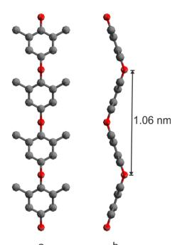
**Fig. 2.2.12** Conformation of PPO chain proposed by imposing tc symmetry, and *c* periodicity 1.06 nm. Projection along *c* axis
