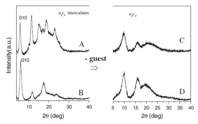
**Fig.1. 3** X-ray diffraction patterns of s-PS films exhibiting  $a_{//}c_{//}$  uniplanar orientation of: A intercalate phase with DMN, B intercalate phase with TMB, C disordered crystalline modification obtained by DMN removal, and D disordered crystalline modification obtained by TMB removal
