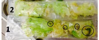
**Fig 2.4.11** Salad iceberg packaging in PP-sPS-PP films: 1) Amorphous 2) crystallized with eco-friendly solvent 3) crystallized with non-eco-friendly solvent. With symbol O maceration is indicated.
