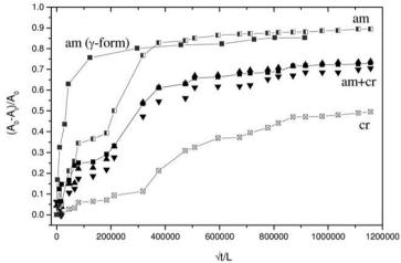
**Fig. 1.17** Carvacrol desorption isotherms, presenting the FTIR absorbance variations  $(A_0-A_t)/A_0$  versus the square root of desorption time divided by film thickness  $(\sqrt{t/L})$ . For comparison, the desorption of carvacrol form the amorphous phase of a  $\gamma$ -form s-PS film is also reported (black squares).
