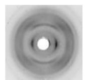
Fig 2.4.10 X-ray diffraction patterns of s-PS films exhibiting the a//c// uniplanar orientation EDGE
