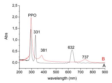
**Fig 4.2.3** UV spectra of PhC with amorphous PPO layers (A)(black line), PhC with crystalline PPO layers (B) (red line)
