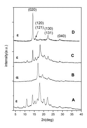
**Fig. 2.3.2.** X-ray diffraction, as collected by an automatic powder diffractometer of PLLA crystalline samples: PLLA/CPO powder (A); PLLA amorphous films immersed in CPO at  $+25^{\circ}$ C (B),  $+2^{\circ}$ C (C), and at  $-25^{\circ}$ C (D) for 3 days. Close to the main diffraction peaks, the Miller indexes of the  $\epsilon$  PLLA co-crystalline phase are indicated.
