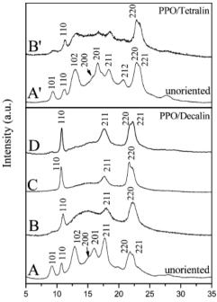
**Fig 2.2.4**. X-ray diffraction patterns, as collected by an automatic powder diffractometer, of PPO/decalin (A–D) and PPO/tetralin (A'–B') cocrystalline samples: (A, A') powders; (B–D) amorphous films exposed to decalin vapor for 24 h at 80 °C (B), 100 °C (C) and 150 °C (D); (B') amorphous film immersed in pure tetralin at room temperature for 1 h. Close to the main diffraction peaks, the Miller indexes are indicated.
