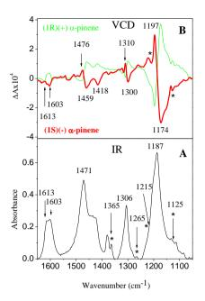
**Fig. 4.3.4** FT-IR (A) and VCD (B) of PPO powders, exhibiting cocrystalline phase with (1R)-(+) $\alpha$ -pinene (thin green line)and (1S)-(-)  $\alpha$ pinene (thick red line) and an  $\alpha$ -pinene content close 30%. The  $\alpha$ -pinene peaks are indicated by a star (\*)<sup>15</sup>
