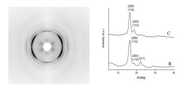
**Fig. 2.3.11.** X-ray diffraction, of  $\alpha$  film presenting uniplanar orientation of the  $\alpha$  crystalline phase. (A) Photographic patterns taken with X-ray beam parallel to the film surface (EDGE pattern). (B-C) Diffraction profiles of photographic patterns taken with X-ray beam parallel (EDGE pattern) (B) or perpendicular to the film surface (THROUGH pattern) (C).
