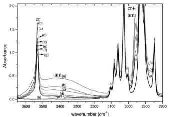
**Fig. 1.15** FTIR transmission spectra in the wavenumber range 3650–2800 cm<sup>-1</sup> of a s-PS/carvacrol co-crystalline film, with an initial carvacrol content close to 40 wt %, as collected at various desorption times (up to 104 hours): (a) t50; (b) 2 days; (c) 20 days; (d) 45 days; (e) 63 days; (f) 157 days; (g) 595 days. FTIR spectra s-PS films nanoporous  $\delta$ -form is also reported (h).
