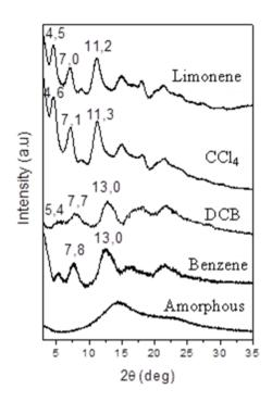
**Fig. 4.3.1** X-ray diffraction, collected by an automatic powder diffractometer. Trend of different nanoporous crystalline phase of PPO obtained by  $CO_2$  extraction of benzene; DCB (1,2-dichlorobenzene); CCl<sub>4</sub>; limonene. For comparison also the PPO Amorphous spectrum is reported.
