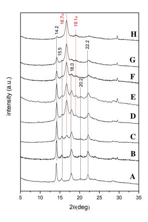
**Fig.2.3.9** Change of X-ray diffraction patterns of  $\varepsilon$ - PLLA/CPO films exhibiting (020) uniplanar orientation (A) with solvent desorption after 7days (B), 16days (C), 26 days (D), 30 days (E), 37days (F), 41 days (G), 69 days (H)
