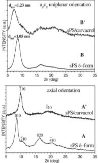
**Fig. 1.9** X-ray diffraction patterns, as taken by an automatic powder diffractometer, of s-PS films exhibiting: (A,B) the  $\delta$  nanoporous-crystalline form with (A) axial orientation and (B)  $a_{//}c_{//}$  uniplanar orientation; (A',B') the sPS/carvacrol  $\delta$ -clathrate form, with (A') axial orientation and (B')  $a_{//}c_{//}$  uniplanar orientation.
