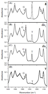
**Fig. 1.6** FTIR spectra of sPS films in the range  $1,400-1,140 \text{ cm}^{-1}$  showing the A nanoporous  $\delta$  phase, B disordered nanoporous crystalline modification obtained from the intercalate phase (dis<sub>i</sub>), C disordered nanoporous crystalline modification obtained from triclinic clathrate phase
