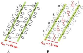
**Fig 1.2** Schematic projections along the chain axis (c axis) showing the crystal structure of: (A) monoclinic nanoporous  $\delta$ -form; (B) monoclinic d clathrate form with carvacrol. High density *ac* layers of closely packed enantiomorphous helices have been pointed out by green ribbons. [Color figure can be viewed in the online issue, which is available at http://wileyonlinelibrary.com.]
