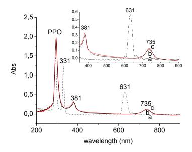
Fig 4.2.5 UV spectra (a) amorphous PPO (dot line); (b) co-PPO\benzene crystal (black line); (c) extracted by  $CO_2$  (red line)
