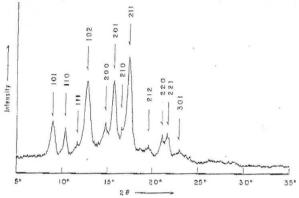
**Fig. 2** X-ray diffraction pattern of chlatrate structure PPO/α-pinene taken from Horikiri S., Journal of polymer Science **1972,**(10), 1167-70
