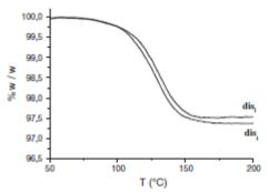
**Fig.1.7** TGA measurements of sPS films in the disordered nanoporouscrystalline modification, obtained from the intercalate phase (dis<sub>i</sub>) and from the triclinic clathrate phase (dis<sub>t</sub>), after DCE equilibrium sorption from 50 ppm aqueous solutions
