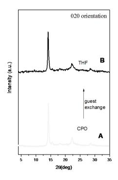
**Fig. 2.3.8** X-ray diffraction patterns of PLLA films: exhibiting (020) uniplanar orientation of the  $\varepsilon$  co-crystalline phase including CPO (A) or THF (B).
