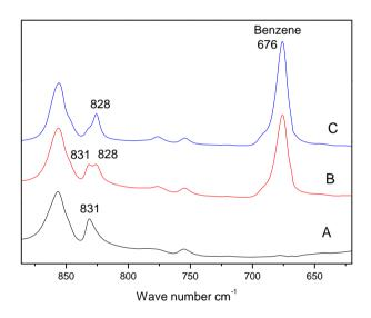
**Fig 4.2.2** FTIR spectra of PhC (or CA/PPO multylayers). A) Amorphous PPO, B) PhC vapours benzene for 15min at 50°C treatment, C) PhC vapours benzene for 30 min at 50°C treatment.
