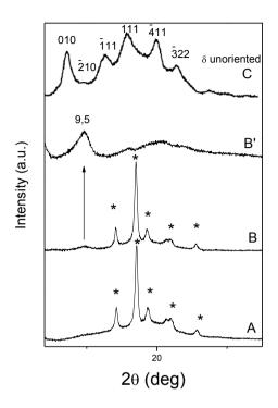
**Fig 2.4.9.** X-ray diffraction of: A) PP-sPS-PP film, B) PP-sPS-PP film after crystallization process (PP signals are indicated with the \*),B') only central sPS film after crystallization process, C) For comparison also unoriented  $\delta$  crystalline phase spectrum is reported
