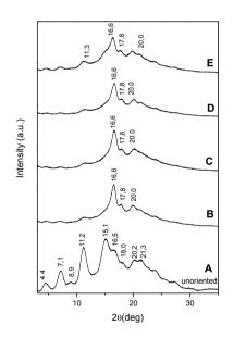
**Fig.2.2.7**. X-ray diffraction, as collected by an automatic powder diffractometer, of PPO/limonene co crystalline samples: (A) powder; (B–E) amorphous films exposed limonene vapor at different temperatures: (B) 70 °C; (C) 80 °C; (D) 120 °C; (E) 160 °C. 20 values are indicated close to the main diffraction peaks.
