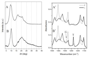
**Fig. 1.8** X-ray diffraction patterns of an axially oriented s-PS film exhibiting the disordered crystalline phase before (A) and after DCE equilibrium sorption from a 50 ppm aqueous solution (B). FTIR spectra, in the range  $1400-1140 \text{ cm}^{-1}$ , taken with the polarization plane parallel (thin line) and perpendicular (thick line) to the stretching direction of films
