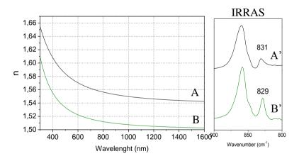
**Fig. 4.3.10** Refractive index n of PPO thin film versus wavelength: A) Amorphou PPO ( black line); B) PPO nanoporous crystalline structure by CCl<sub>4</sub> (green line). The respective IRRAS spectra (A'-B') are reported
