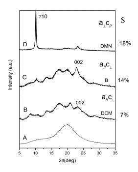
**Fig.2.4.3** X-ray diffraction collected by an automatic powder diffractometer of uniplanar orientation of  $\delta$  *co*-crystalline phases including DCM (B), B(C) and DMNP (D) guest molecules. The orientations can be defined as  $a_{l/C\perp}$ , (B-C) and  $a_{\perp Cl'}$  (D) uniplanar ; for sake of comparison the amorphous is also reported (A) and shrinkage values (S) are also indicated
