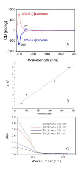
**Fig. 3. 9.** (A) CD spectra of film (thickness 300 nm), after (R)-(-) carvone (red thin line) or (S)-(+) carvone (blue thick line) induced crystallization; (B) Degree of circular polarization as a function of film thickness for sPS spin-coated films; (C) UV Absorbance spectra of sPS spin-coted films.
