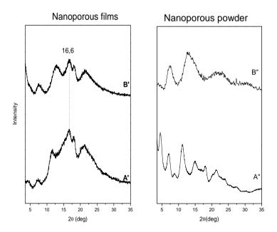
**Fig. 2.2.11** (A) oriented PPO/limonene film emptied with CO<sub>2</sub>; (B) oriented PPO/tetralin film emptied with CO<sub>2</sub>; (A') PPO/limonene powder emptied with CO<sub>2</sub>; (B') PPO/tetralin powder emptied with CO<sub>2</sub>
