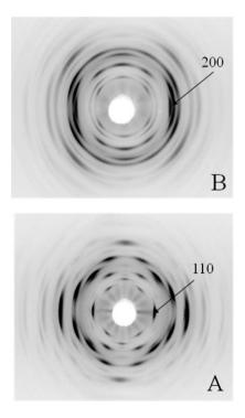
**Fig. 2.2.3**. Photographic X-ray diffraction patterns, obtained with X-ray beam parallel to the film plane (EDGE), of amorphous films crystallized by exposure to  $\alpha$ -pinene vapor, whose patterns as collected by an automatic powder diffractometer are shown in Figure 2, parts E (A) and F (B). The Miller indexes of the most intense equatorial peaks are indicated.
