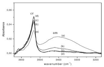
**Fig 1.12** FTIR transmission spectra in the wavenumber range 3650–3150 cm<sup>-1</sup> of a  $\delta$ -form s-PS film, after equilibrium sorption from a 5 wt % carvacrol solution in acetone, as collected at various desorption times: (a) 1 hour; (b) 24 hours; (c) 155 hours; (d) 395 hours.
