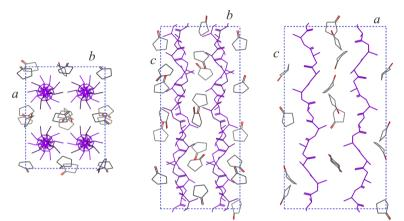
**Fig. 2.3.6.** Schematic representation of the proposed crystalline PLLA-CPO clathrate form in projection along the c axis, a axis and b axis. 10/7 helical chains are reported in magenta. Guest molecules are arranged in isolated elements characterized by a complex shape presenting their main axis parallel to the c axis of the unit cell.
