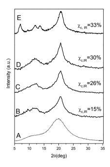
**Fig 2.4.4** X-ray diffraction patterns of s-PS films annealed at different temperatures: (A), mesomorphic trans-planar (B-D) obtained by annealing amorphous films at 130°C for 1h (B),2h(C) 3h(D), and crystalline  $\alpha$  form films (E), and different crystallinity degree ( $\chi_c$ ) is indicated
