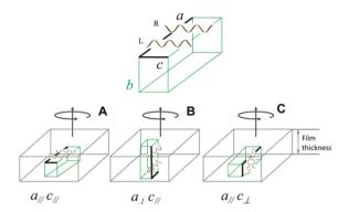
**Scheme 2. 1**. Schematic Presentation of the Three Uniplanar Orientations of s-PS Cocrystalline Films, Corresponding to the Three Simplest Orientations of the High-Planar-Density ac Layers with Respect to the Film Plane
