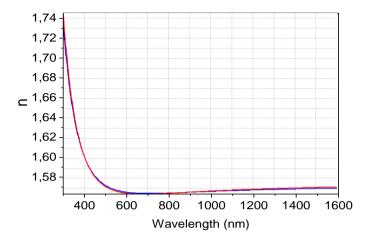
Fig.4.3.8 Refractive index n of amorphus PPO thin film versus wavelength
