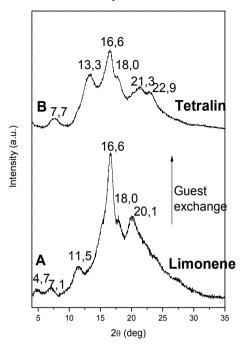
**Fig. 2.2.10**. X-ray diffraction patterns of PPO films: (A) exhibiting  $00\ell$  orientations of the cocrystalline phase with limonene; (B) after exchange with tetralin;
