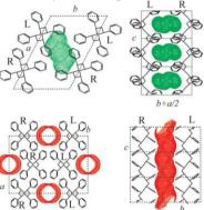
**Fig.1** Top and lateral views of the crystalline structures of the two nanoporous crystalline forms of s-PS. For the  $\delta$  (upper figures) and  $\epsilon$  (lower figures) forms, the porosity is distributed as cavities and channels, respectively.<sup>4</sup>
