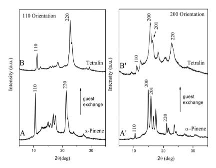
**Fig. 2.2.5**. X-ray diffraction patterns of PPO films: (A, A') exhibiting two different uniplanar orientations of the cocrystalline phase with  $\alpha$ -pinene, 110(A) or 200 (A'); (B, B') as obtained by  $\alpha$ -pinene exchange with tetralin (retention of uniplanar orientations).
