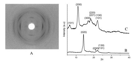
**Fig. 2.3.4.** X-ray diffraction, of  $\varepsilon$  PLLA/CPO film presenting (020) uniplanar orientation. (A) Photographic patterns taken with X-ray beam parallel to the film surface (EDGE). (B-C) Diffraction profiles of photographic patterns taken with X-ray beam parallel (EDGE) (B) or perpendicular to the film surface (THROUGH) (C).
