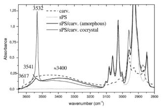
**Fig.1.10** FTIR spectra of s-PS films presenting: (thin dotted line) nanoporous  $\delta$ -form; (thin full line)  $\delta$  clathrate form with carvacrol and (thick full line)  $\lambda$ -form. The FTIR spectrum of liquid carvacrol is shown as a thick dashed line.
