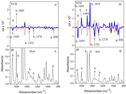
**Fig 3.2.** FTIR (A, B) and VCD spectra (A', B') of amorphous s-PS films, having a thickness of nearly 20  $\mu$ m (A, A') or 6  $\mu$ m (B, B'), after crystallization induced by sorption of (R)-(-) carvone (thin red line) or (S)-(+) carvone (thick blue line). The main peaks of the carvone guest are labeled by "g" while some typical peaks of the polymer host are indicated by "h".
