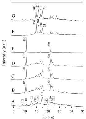
**Fig 2.2.2** X-ray diffraction, as collected by an automatic powder diffractometer, of PPO/ $\alpha$ -pinene cocrystalline samples: (A) powder; (B–G) amorphous films exposed to  $\alpha$ -pinene vapor at different temperatures: (B) 110 °C; (C) 120 °C; (D) 130 °C; (E) 140 °C; (F) 150 °C; (G) 160 °C. Close to the main diffraction peaks, the Miller indexes are indicated.
