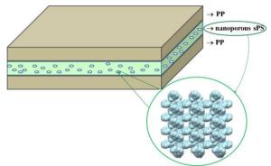
**Fig. 2.4.8** Multilayer film based on the common PP and including a core layer of nanoporous syndiotactic polystyrene (s-PS).
