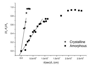
**Fig. 4.3.7** CCl<sub>4</sub> desorption isotherms, presenting the FTIR absorbance variations  $(A_0-A_1)/A_0$  versus the square root of desorption time divided by film thickness  $(\sqrt{t/L})$ . For comparison, CCl<sub>4</sub> desorption from amorphous phase and from crystalline phase of PPO, is reported.
