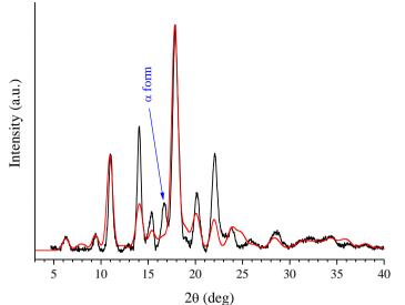
**Fig. 2.3.7** Comparison between experimental (black line) X-ray powder diffraction pattern for the PLLA-CPO clathrate form, after the subtraction of the amorphous contribution, with the calculated one (red line) according to the structural model reported in Figure 2.3.6.
