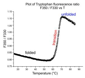
Figure 1.6.3: nanoDSF principle.
