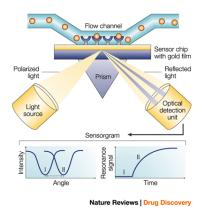
Figure 1.6.1: Typical set-up for a Surface Plasmon Resonance biosensor<sup>48</sup>.
