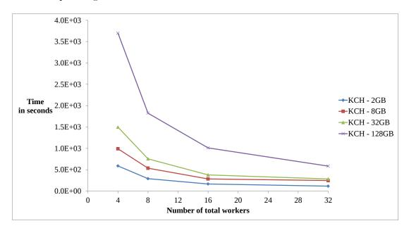
Figure 5.19: KCH Local Statistics. Scalability of KCH, for the case k = 7, for all datasets, which are indicated in the figure according to the legend to the right. The abscissa gives the number of workers used, while the ordinate gives the corresponding time.
