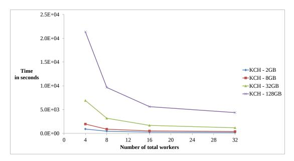
Figure 5.25: KCH Cumulative Statistics. Scalability of KCH, for the case k = 31, for all datasets, which are indicated in the figure according to the legend to the right. The abscissa gives the number of workers used, while the ordinate gives the corresponding time.
