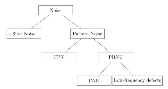
Figure 4.1: The components of the noise in a digital image.
