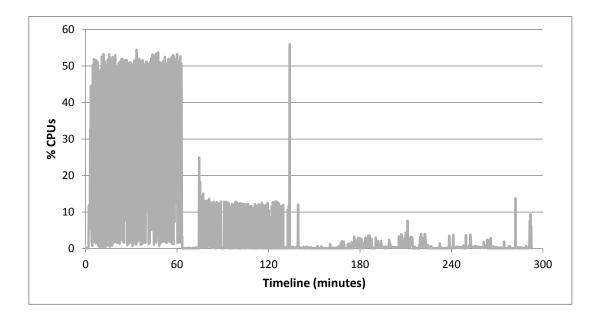
Figure 4.8: CPU usage of *slave1*, in percentage, when running Step I of HSCI\_Seq.
