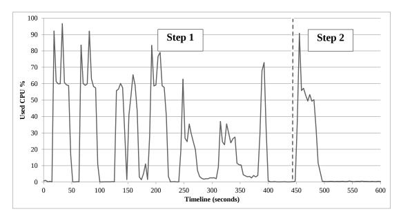
Figure 5.8: CPU usage profile of a slave node of the Hadoop cluster used for evaluating the Squared Euclidean dissimilarity between 20 different sequences of  $\approx 1,600,000,000$  characters each, with k = 10 and 8 concurrent map/reduce tasks on each slave node (*i.e.*, 32 total workers). For gathering information, we used Dstat tool [293].
