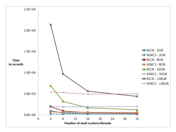
Figure 5.29: Cumulative Statistics. Scalability of our algorithm (KCH) with respect to KMC2, for the case k = 31 and for all datasets, which are indicated in the figure according to the legend to the right. The abscissa indicates the number of workers/threads used, while the ordinate gives the corresponding time in seconds.
