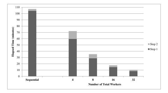
Figure 5.7: Elapsed times for evaluating the Squared Euclidean dissimilarity measure between 20 different sequences of  $\approx 1,600,000,000$  characters each, with k = 10 and an increasing number of concurrent map/reduce tasks at the same time (*i.e.*, workers or Hadoop Containers).
