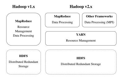
Figure 3.2: The software architectural difference between Hadoop v1.x and v2.x.
