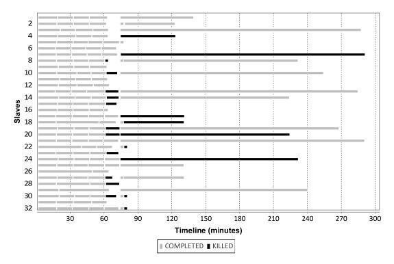
Figure 4.7: HSCI\_Seq variant - An overview of map and reduce tasks launched during an execution of Step I. Notice that reduce tasks start only after the termination of all map tasks as described in Section 4.4.2.3.
