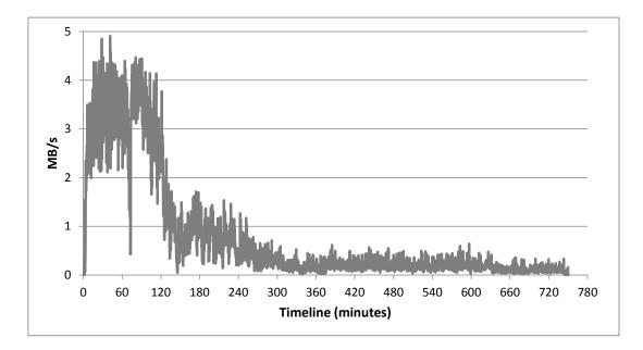
Figure 4.6: Average incoming network throughput, in MB/s, when running Step I of  $\tt HSCI.$
