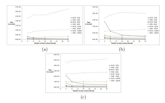
Figure A.3: Cumulative Statistics. (a) Scalability of KCH with respect to DSK, for the case k = 7, for all datasets, which are indicated in the figure according to the legend to the right. The abscissa gives the number of workers/threads used, while the ordinate gives the corresponding time in seconds. (b)-(c) As in (a), but for k = 15 and k = 31, respectively.
