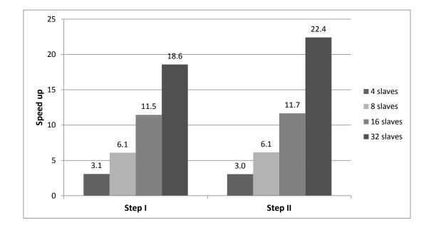
Figure 4.16: Speed up of HSCI\_All compared to SCI when running on a cluster of increasing size.
