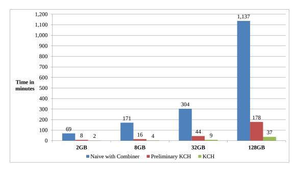
Figure 5.14: Cumulative Statistics. Comparison of KCH versus the Hadoop-based naive solution with Combiner and Preliminary KCH using k = 15 for all datasets.
