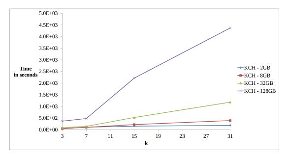
Figure 5.26: KCH Cumulative Statistics. Execution times of KCH for the all datasets and for k = 3, 7, 15, 31 using 32 total workers.
