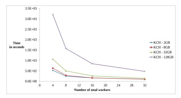
Figure 5.23: KCH Cumulative Statistics. Scalability of KCH, for the case k = 7, for all datasets, which are indicated in the figure according to the legend to the right. The abscissa gives the number of workers used, while the ordinate gives the corresponding time.
