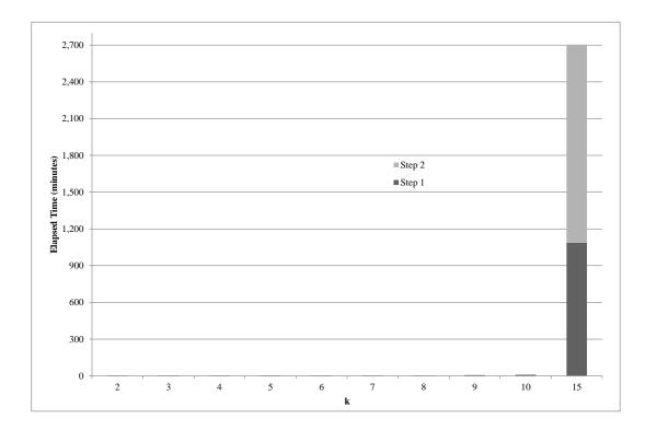
Figure 5.9: Elapsed times for evaluating the Squared Euclidean dissimilarity between 20 different sequences of  $\approx 1,600,000,000$  characters each, using 32 concurrent workers, and values of k increasing up to 15.
