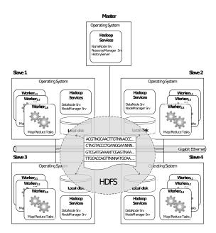
Figure 5.13: A schematic representation of a cluster configured to run KCH algorithm designed for Hadoop. The communication among nodes uses the Gigabit Ethernet, while the storage of input and output files is distributed among the local disks present in each slave node.
