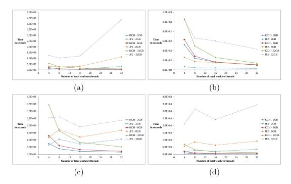
Figure A.4: Cumulative Statistics. (a) Scalability of KCH with respect to Jellyfish, for the case k = 3, for all datasets, which are indicated in the figure according to the legend to the right. The abscissa gives the number of workers/threads used, while the ordinate gives the corresponding time in seconds. (b)-(d) As in (a), but for k = 7, k = 15 and k = 31, respectively.
