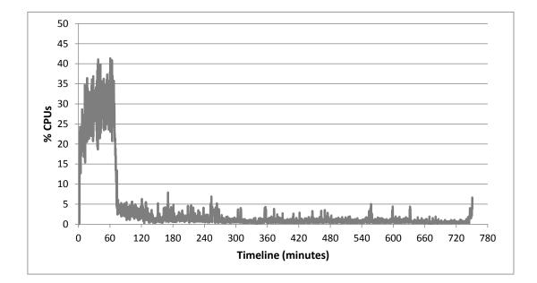
Figure 4.5: Average CPU usage of slave nodes, in percentage, when running Step I of HSCI.
