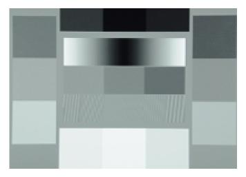
Figure 4.3: An example of enrollment image. The scene is from a test chart used for noise measurements, ISO 15739 [223].
