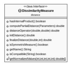
Figure 5.3: The Java Interface DissimilarityMeasure used in our framework to manage a dissimilarity measure for alignment-free sequence comparison.
