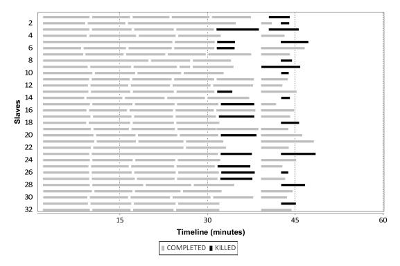
Figure 4.15: HSCI\_All variant - An overview of map and reduce tasks launched during Step I. Notice that reduce tasks start only after the termination of all map tasks as described in Section 4.4.2.3.
