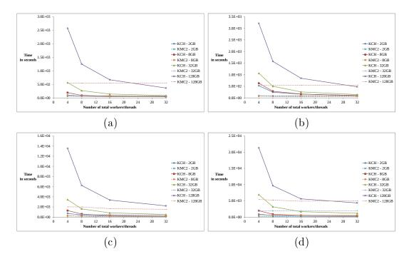
Figure A.2: Cumulative Statistics. (a) Scalability of KCH with respect to KMC2, for the case k = 3, for all datasets, which are indicated in the figure according to the legend to the right. The abscissa gives the number of workers/threads used, while the ordinate gives the corresponding time in seconds. (b)-(d) As in (a), but for k = 7, k = 15 and k = 31, respectively.
