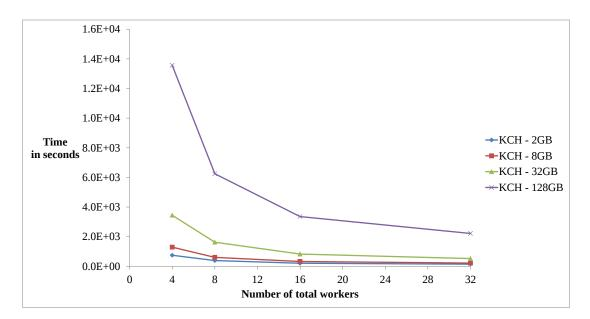
Figure 5.24: KCH Cumulative Statistics. Scalability of KCH, for the case k = 15, for all datasets, which are indicated in the figure according to the legend to the right. The abscissa gives the number of workers used, while the ordinate gives the corresponding time.
