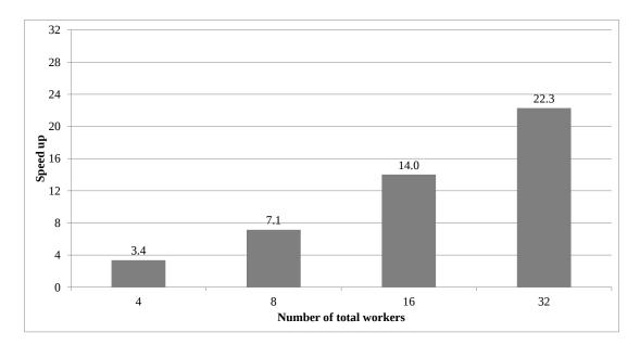
Figure 5.28: KCH Cumulative Statistics. Speed up of KCH for the case k = 15 and dataset  $CS\_32GB$ . The abscissa gives the number of workers used, while the ordinate gives the corresponding speed up than our stand-alone implementation executed on a single-core.
