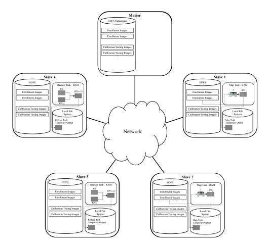
Figure 4.2: Conceptual view of our distributed algorithm for SCI when running the Step I on a cluster of 4 slave nodes. Images are not centralized but they are saved on HDFS. Slave 1 and Slave 2 are extracting RNs from enrollment images available on HDFS (map task). The result of this extraction can be buffered on local file system before being sent to HDFS. Slave 3 and Slave 4 are summing and averaging all RNs of images shot using a same camera to compute the RP(reduce task).
