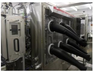
**Figure 3.5** - Kurt J. Lesker Company evaporator system incorporated in a Jacomex glove box used for metal evaporations
