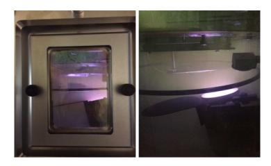
**Figure 5.1** - Plasma discharge in Argon in the Kurt J. Lesker sputtering system used for RF sputtering deposition of Al<sub>2</sub>O<sub>3</sub>.
