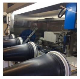
Figure 3.6 - Nordson EFD automatic dispenser used for resin dispensation included in an MBRAUN glove box
