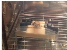
**Figure 3.4** - Votsch climate chamber utilized for Electrical Calcium Test conditionings and measurement station for accommodation of the sample
