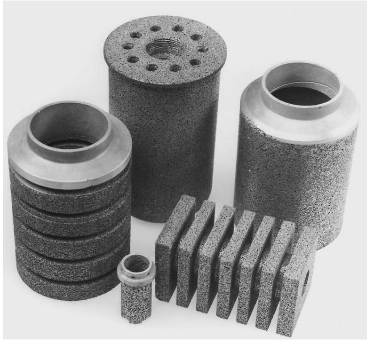
Figure 9 Mechanic structure made by metallic foam (Banhart J., 2001)
