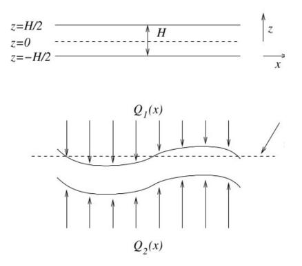
Figure 2.15: (a) Elastic lamina of thickness H in initial conditions with no stresses; (b) Elastic lamina after the application of stress load  $Q_1(x)$  and  $Q_2(x)$
