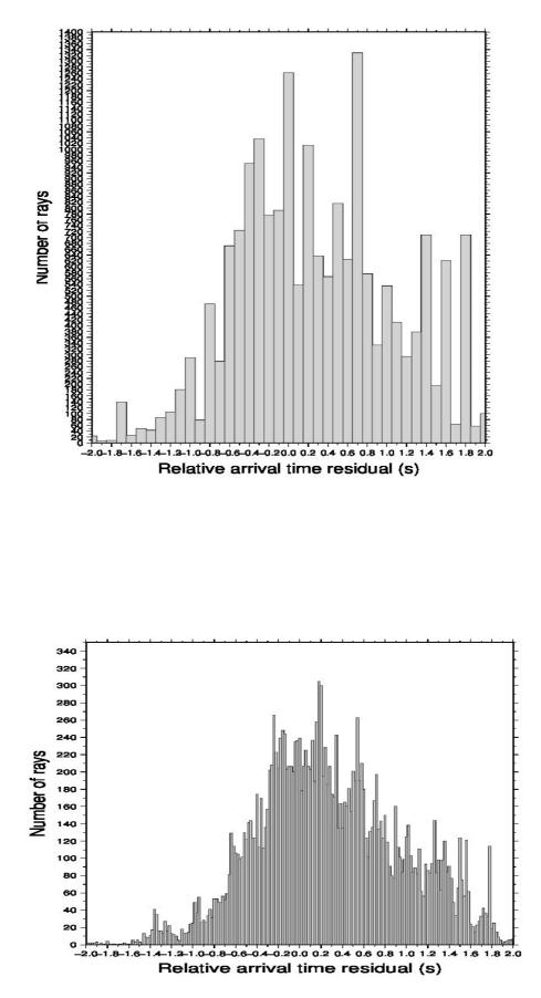
Figure 4.5: Histograms of relative arrival time residuals of observed traveltimes for initial model (up) and final model after six iterations (down)
