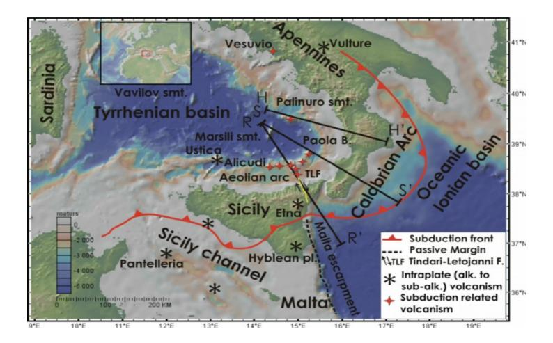
Figure 4.1: Schematic geological map of Southern Italy ("Seismic velocity structures of Southern Italy from tomographic imaging of Ionian slab and petrological interferences", Calò et al., 2012)
