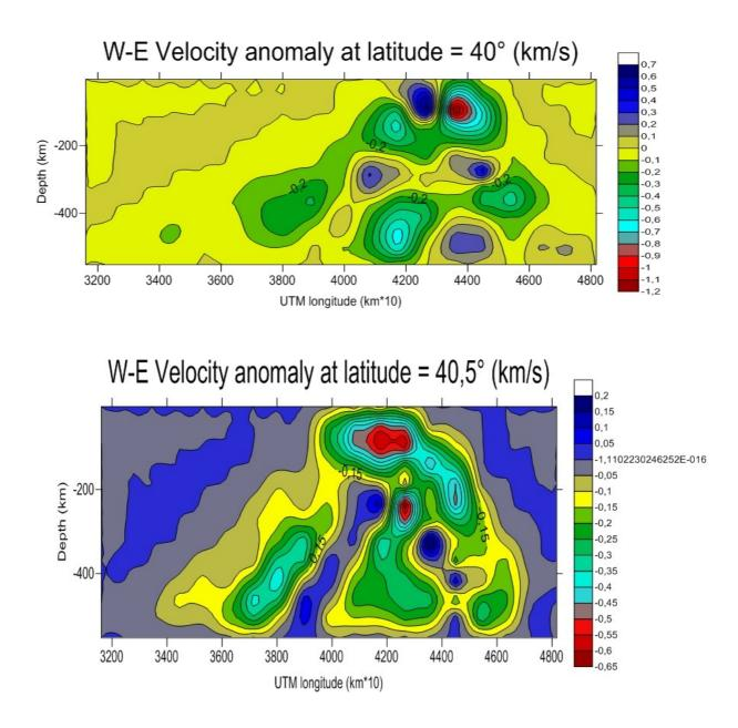
Figure 4.10: Vertical sections WE of velocity anomaly made by Golden Surfer at fixed latitude of 39°, 39.5°, 40° and 40.5°
