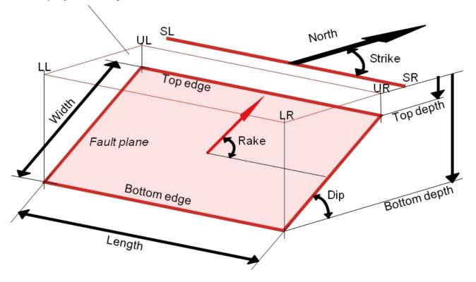
Figure A.2.1: Scheme of a fault and of its characteristics
