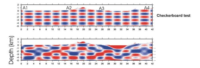
Figure 1.5: example of checkerboard test for a seismic tomography
