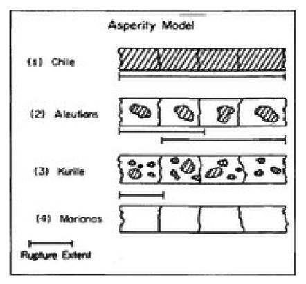
Figure 2.12: Schematic diagram of the asperity model for stress heterogeneity on the fault plane (Lay & Kanamori, 1981)
