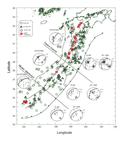
Figure 2.11: Illustration of earthquakes and of focal mechanisms in double Northern Japan Wadati-Benioff zones
