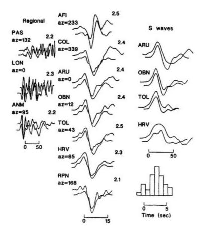
Figure 3.7: An example of waveform modeling for the 1989 Loma Prieta earthquake. Ground displacements are for the P<sub>n</sub> and teleseismic P and SH waves ("A broadband seismological investigation of the 1989 Loma Prieta, California earthquake; evidence for deep slow slip?", Wallace et al.,, 1991)
