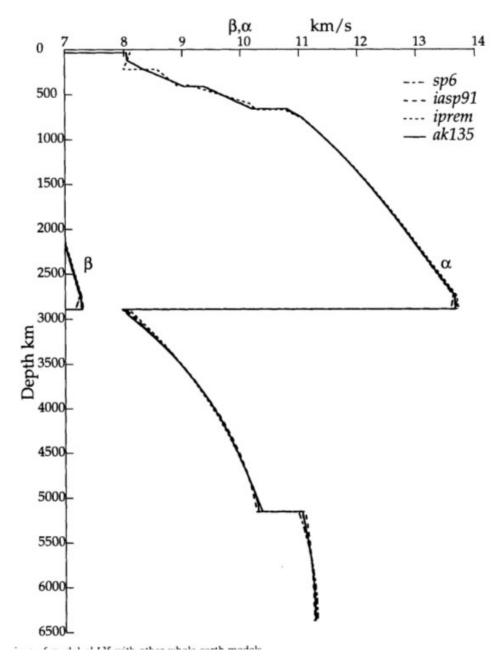
Figure A.1.3: Comparison of model ak135 for both P and S wavespeeds (respectively, α and β) with other 1-D velocity models (from "Constraints on seismic velocities in the Earth from traveltimes", Kennett, Engdahl & Buland, Geophys. J. Int (1995), 122, 108-124)
