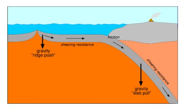
Figure 2.8: Illustration of "ridge push" and of "slab pull"
