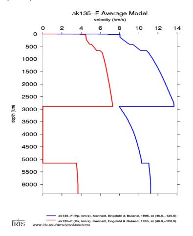
Figure 1.4: ak153 1D velocity model (blue for P waves, red for S waves)
