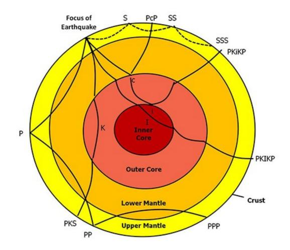
Figure 3.4: Graphical representation for various surface reflections observed in the Earth and raypaths for various core phases
