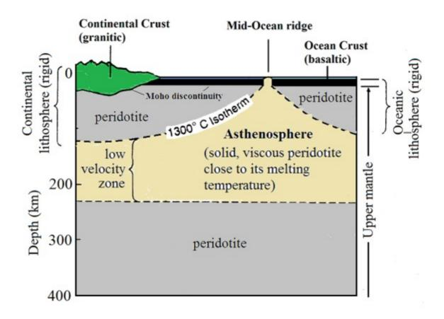
Figure 2.1: schematic stratigraphy of lithosphere and astenosphere
