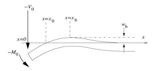
Figure 2.16: Elastic lamina where on it acts a load  $V_{0}\,and$  a flexing momentum  $M_{0}$
