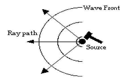
Figure A.2.2: Geometric scheme of a seismic raypath
