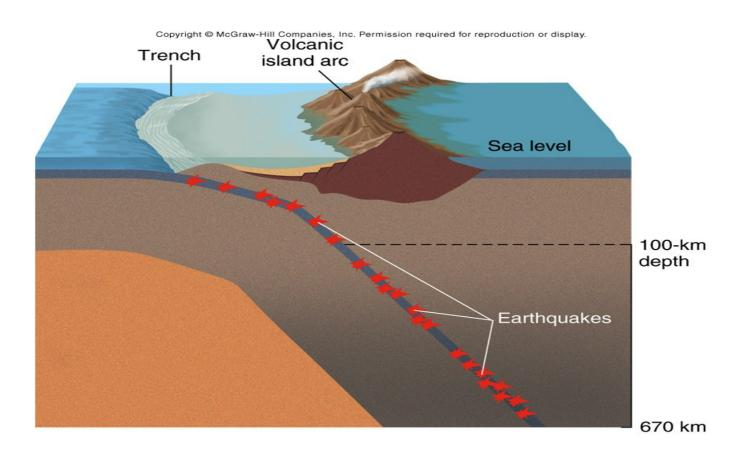
Figure 2.9: Illustration of a Wadati-Benioff zone with earthquakes distributed along a subduction slab
