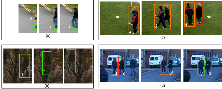
Figure 3.9 Output of the tracking algorithm based on the proposed FSA, when applied to the problems discussed in Section 3.2. (a) The entering object is correctly recognized as a single object, and not a group. (b) The object identity is preserved when the person passes behind the tree. (c) A group initially classified as a single person is correctly handled when classification becomes stable. (d) The group object maintains the constituent object identities.
