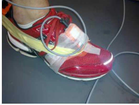
Figure 2.5 A foot mounted IMU. Taken from http://www.wearable.ethz.ch
