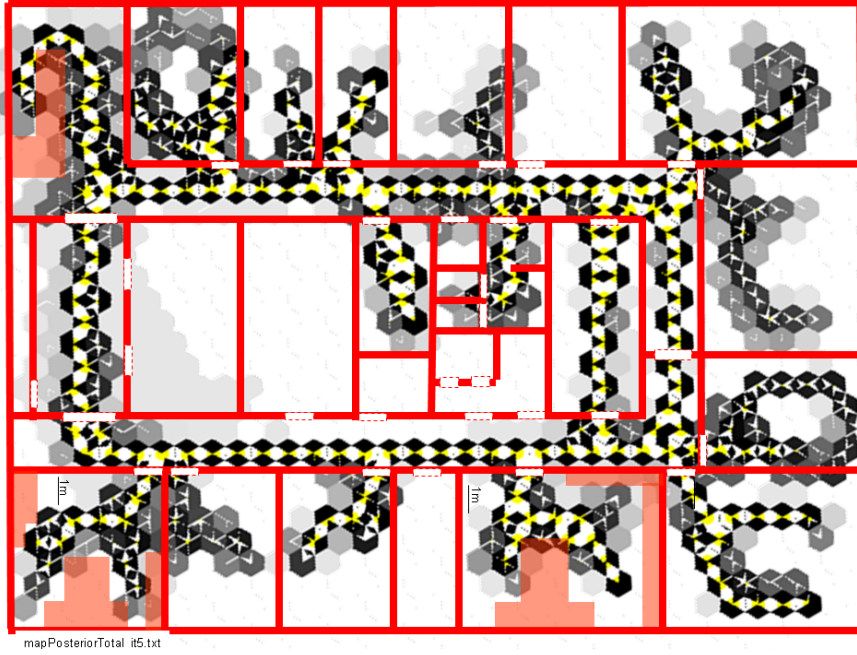
Figure 5.5 Map processed by FeetSLAM, derived from 4 independent maps obtained through FootSLAM. The elaboration is offline, and encompasses only the best particle.
