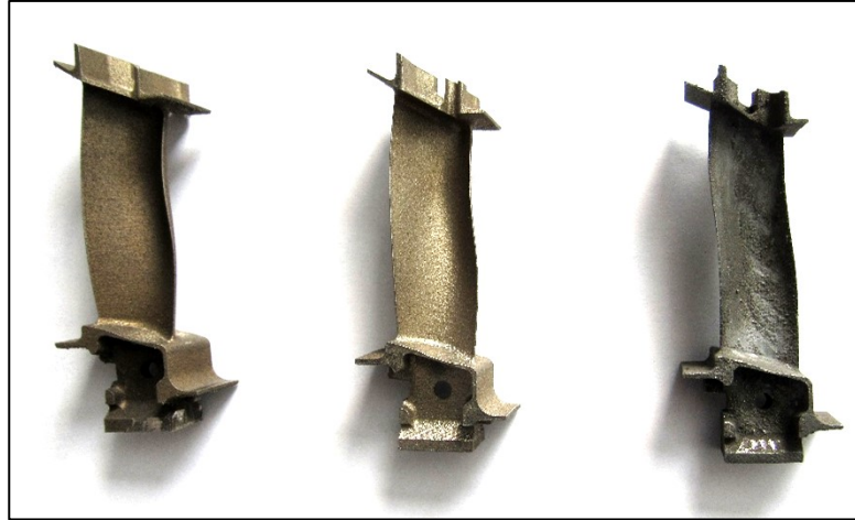
Figure 2.14: Flat-, 45°- and upright-built turbine blade, removed from the building plate, heat treated
