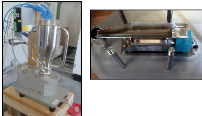
Figure 3.5: Medicoat vibrating powder system and oscillating channel
