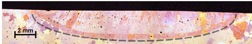
Figure 3.34: Longitudinal cross-section of the groove upon repairing and milling of the allowance
