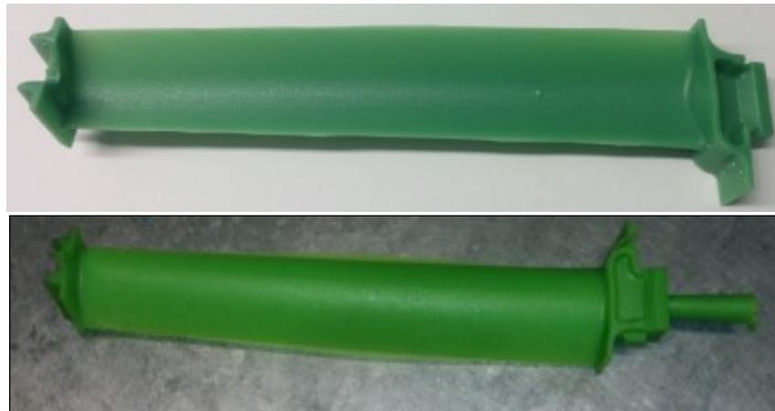
Figure 1.29: wax blades casting with AM mould
