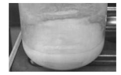
Figure X.1: Monolith dipped in the washcoat.
