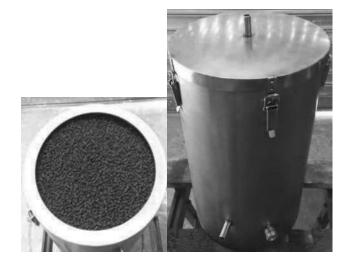
Figure VI.10: Activated carbon for H<sub>2</sub>S residual removal by adsorption.
