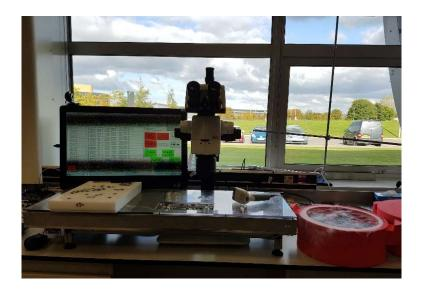
**Figure 4.7** The Shifter: a microscope x-y stage that also handles the unsealing and the resealing as well as the automatically samples tracking
