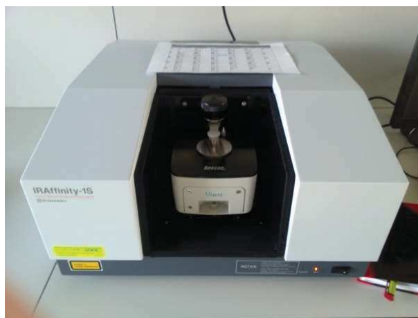
Figure 3.5: FT-IR instrument equipped with the ATR FTIR accessory.
