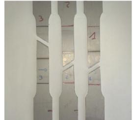
Figure 5.19 – Welded specimens after tensile tests
