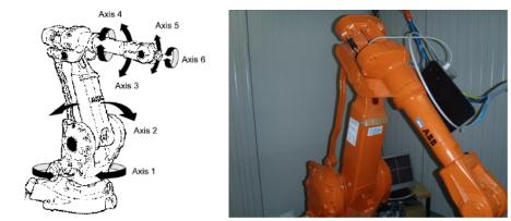
Figure 4.5 – Robot ABB IRB 2400
