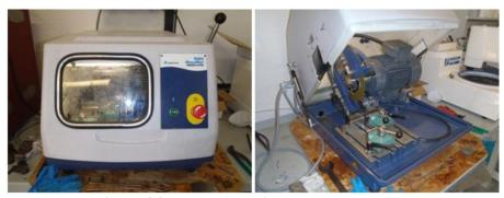
Figure 4.8 – Delta AbrasiMet bench-top cutter
