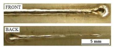
Figure 4.18 – BoP at 1400 W, 100 mm/s and -2 mm
