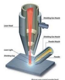
Figure 3.1 – Laser welding process
