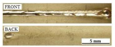
Figure 4.17 – BoP at 1400 W, 110 mm/s and -2 mm
