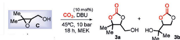
Scheme 5.6. Reaction of a trisubstituted epoxide ( C ) and CO_2 into its respective cyclic carbonates.
