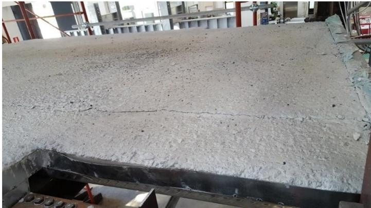
**Fig. 5.183** - Collapse of the slab
