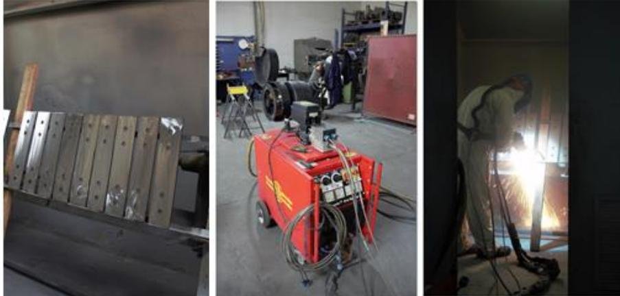
**Fig. 2.3** – Electric arc wire spray: a) plates before spray; b) machine for electric arc wire spray; c) spray coating.
