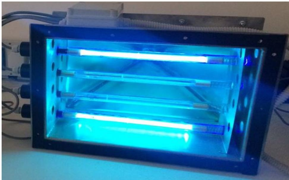
Figure 7-3: UV lamps configuration
