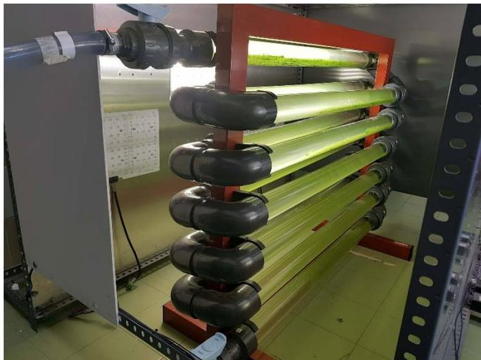
*Figure 7-7: Tubular Photo-Bioreactor*
