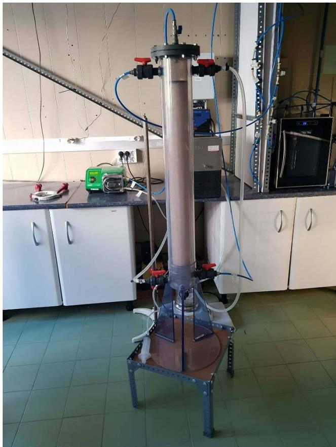
*Figure 7-6: Biotrickling filter*
