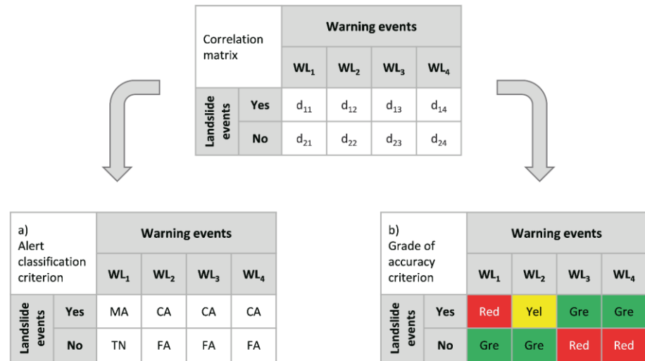
Figure 6.13 Alert classification (a) and grade of correctness (b) performance criteria used for the analysis of the correlation matrix (modified from Calvello and Picullo 2016 )
