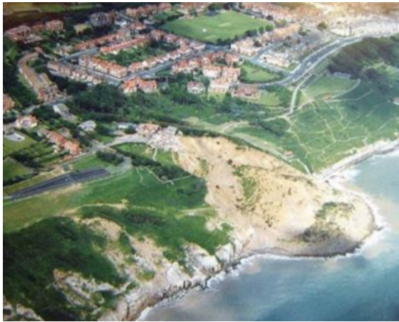
Figure 2.9 Coastal landslide occurred in Scarborough, south-eastern coast of England (McInnes and Moore 2011)
