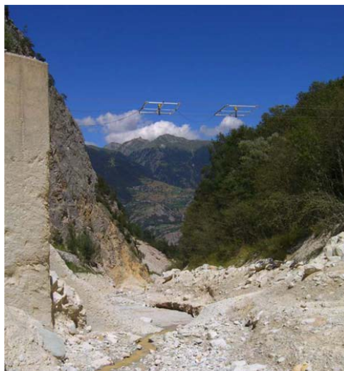
Figure 2.22 Downstream view of two radar sensors for measuring flow depth as employed in the Illgraben catchment ( Badoux et al. 2009 )
