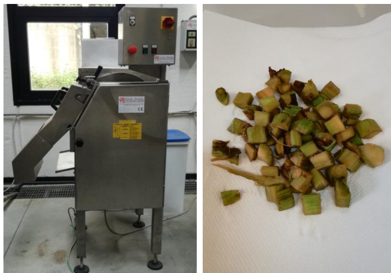
Figure III.4 Picture of the pilot dicer machine available at laboratories of ProdAl S.c.a.r.l (left) and artichoke stem cubes used in the experimental campaign (right).
