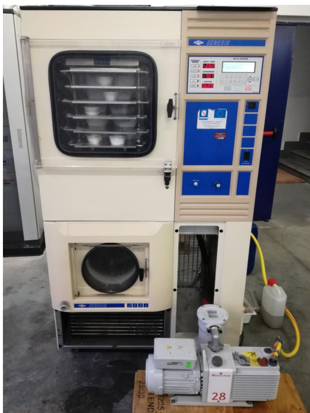
Figure III.10 Picture of freeze-drier used for the obtainment of solid extracts from artichoke waste retentate stream.
