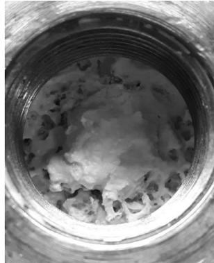
**Figure III.17** Photographs of foaming materials in the saturator.
