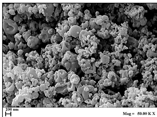
**Figure IV.35.** FESEM image of HP $\beta$ CD micronized by SAA technique.
