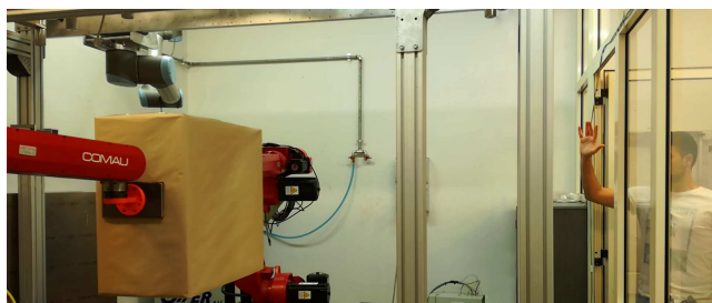
Figure 3.12: Experimental case study. Representation of the cooperative transportation task by the Comau robots. A human operator (on the right) moves nearby and his right hand is selected as representative point.
