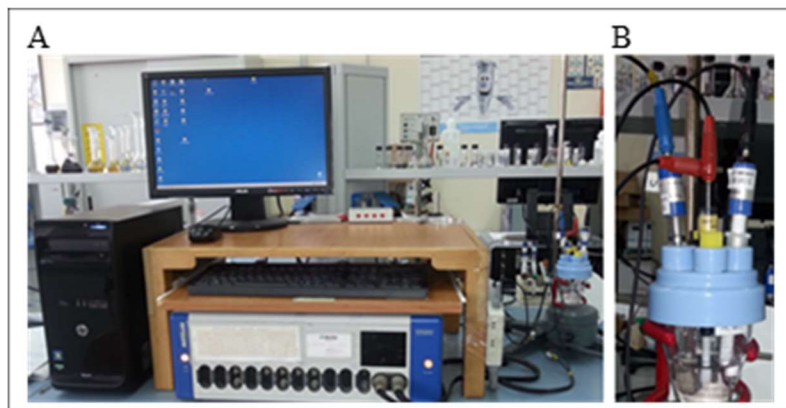
Figure 3.1: PGSTAT 30 potentiostat / galvanostat with measurement cell and acquisition system.
