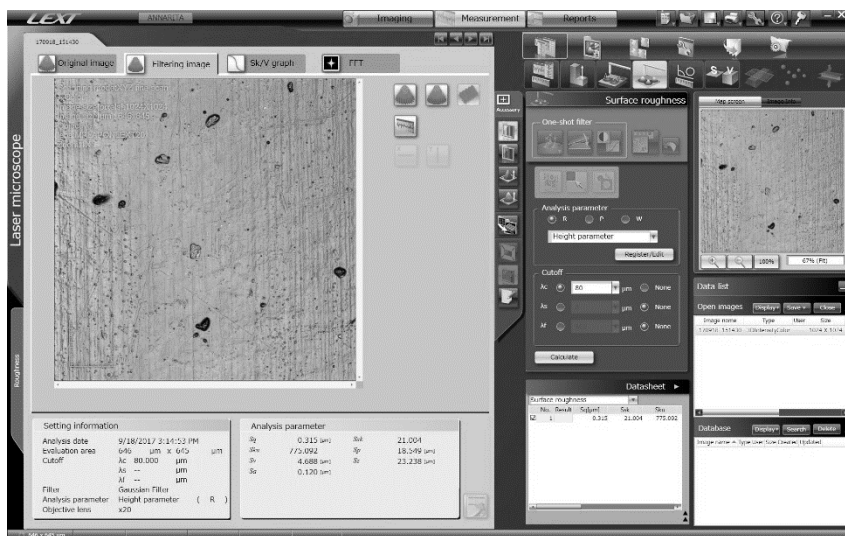
Figure 78. Surface mapping of the area close to the gate of the micro-injection molded part.
