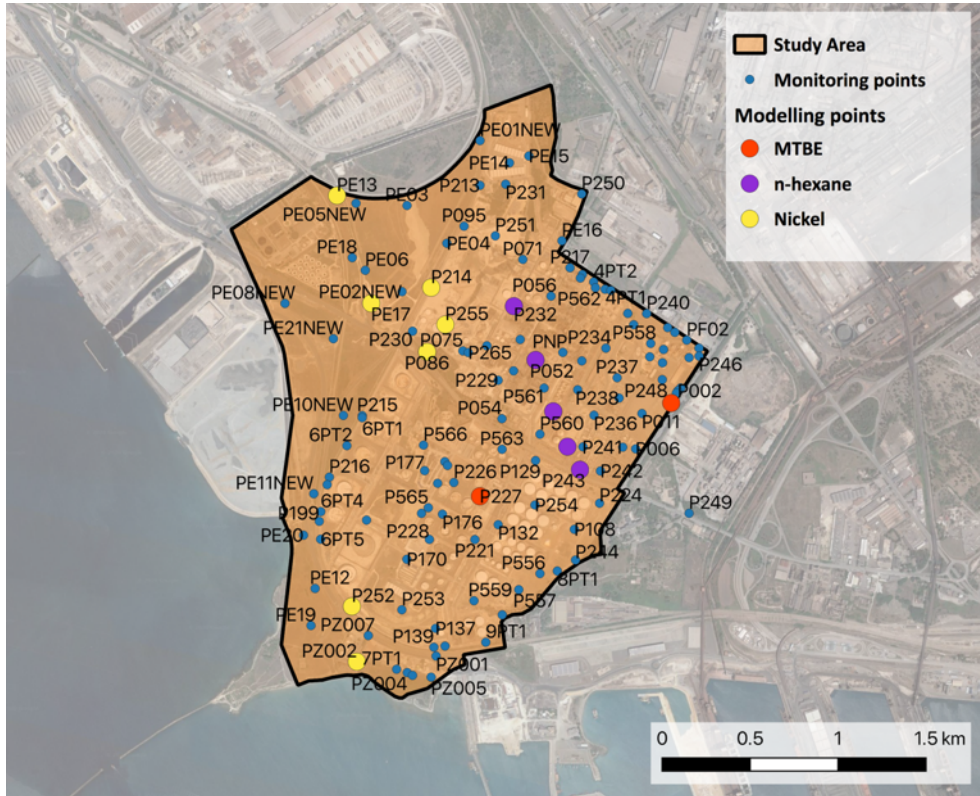
Figure 7.5: Location of modelling points with the considered contaminant in the study area
