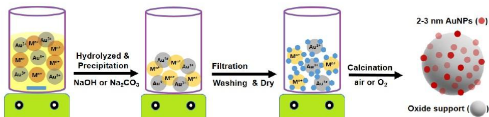
Figure 22: preparation of AuNPs via Co-Precipitation method.
