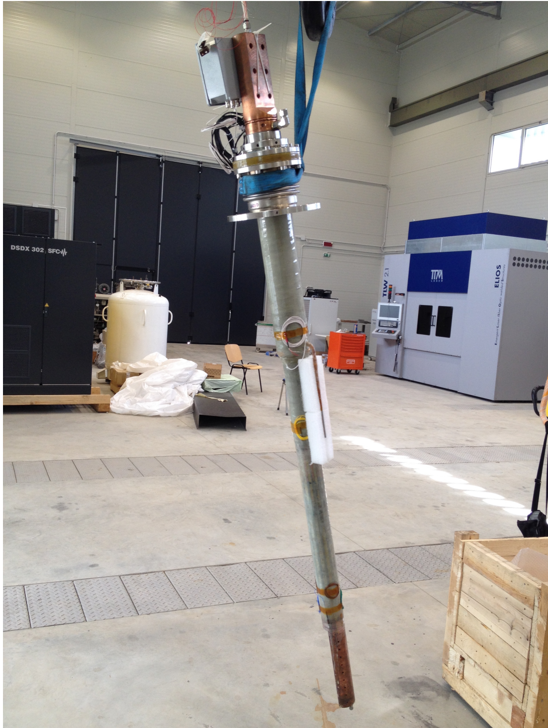
Fig.3.14 Picture of one of the HTS current leads with a total length of 1700 mm.
