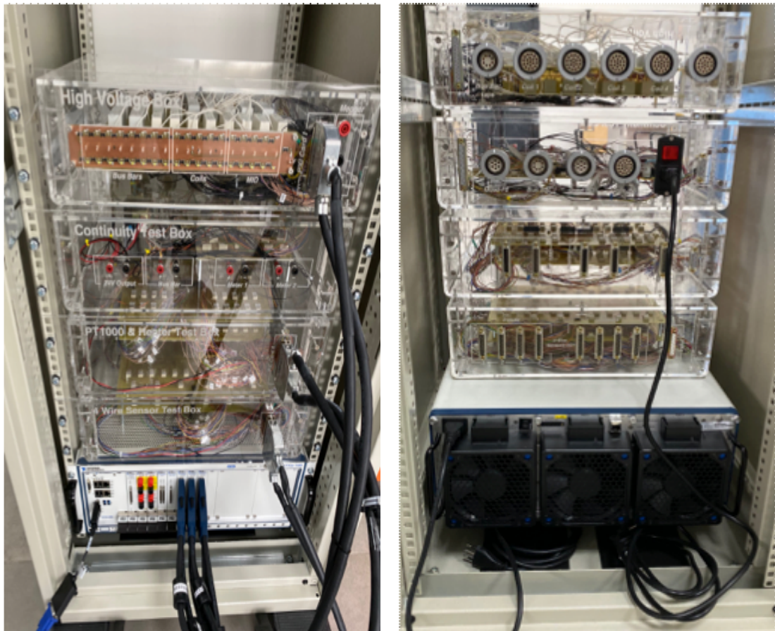
Fig.4.17 The automatic QDM test system front (left) and back view (right). Under the last switch box on the bottom of both figures, there is a PXI computer that manages the switch boxes and all the other instruments.
