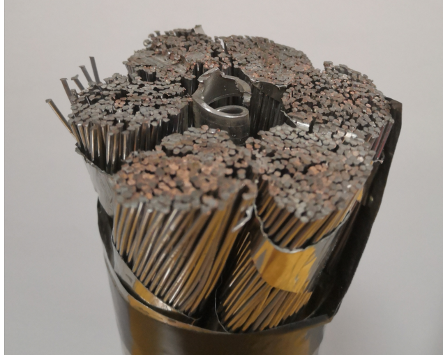
Fig.1.03 Cross-section of the 1080 strands on a CICC cable of the ITER coil.
