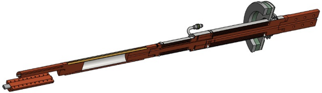
Fig.3.12 CAD design of the complete HTS current lead with its superconducting part, shown by the gray-colored zone under the yellow line with its two copper clamps. The Liquid nitrogen input pipe to the reservoir is also visible. The overall length of the current lead is about 1.7 meters.
