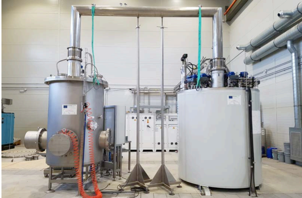
Fig.4.11 The LR280R cryogenic refrigerator, produced by Linde Kryotechnik, is connected to the Cold-Box through the cryogenic transfer pipe.
