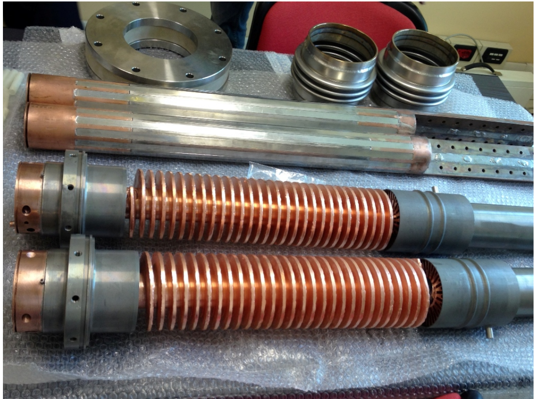
Fig.3.13 Picture of the main parts of the two HTS current leads before the final assembly. The superconducting parts with their soft soldered (2G) ReBCO superconducting strips (Top). The copper made, gas exchangers showing the cooling path of the cold nitrogen gas obtained from the evaporation of the liquid nitrogen of the reservoir (Bottom).
