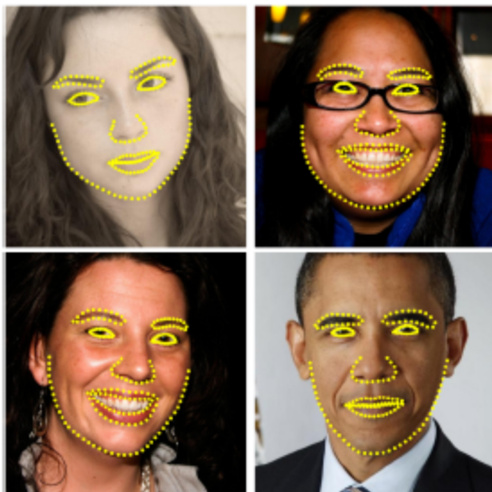
Figure 4.19: Face Detector (Dlib) is the result of applying a set of random regression trees, used to extract 194 landmarks of a face in an image.
