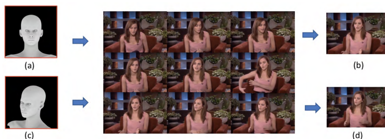
Figure 2.19: Search for the desired pose in a sequence of frames extracted from a video interview (a) Search for an image that matches the frontal pose (the one with angle P: +00^\circ , Y: +00^\circ , R: +00^\circ ) (b) Front-most frame in the sequence (c) Search for an image that matches pose with angles: P +10^\circ , Y +30^\circ , R +05^\circ (d) Frame more similar to the required pose.
