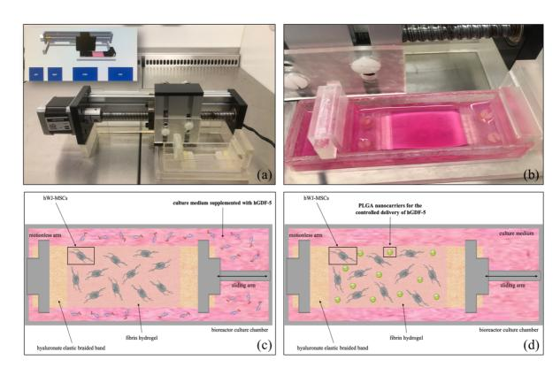
**Figure 5-4.** Cyclic strain bioreactor and experimental design (a) Image of the cyclic strain bioreactor and software interface. (b) 3D scaffold placed in the bioreactor culture chamber. Two series of experiments were performed: (c) hGDF-5 was supplemented in the culture medium or (d) encapsulated within PLGA carriers for growth factor controlled delivery.
