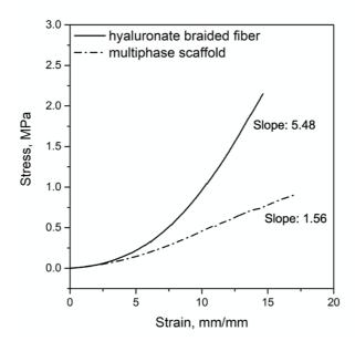
**Figure 5-3. Mechanical characterization of the 3D scaffold.** Stress–strain plot and elastic modulus values (a) and maximum load (b) of hyaluronate braided band (continuous line) and of multiphase stem cell-based scaffold (dashed line).
