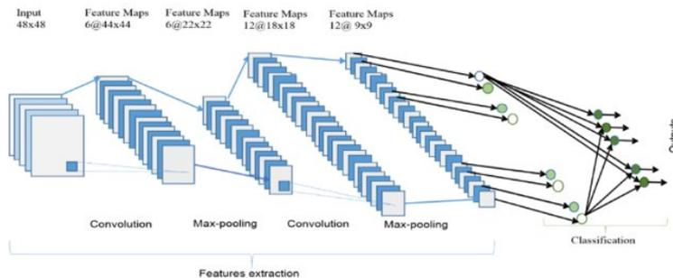
Figure 2.3: CNN architecture.
