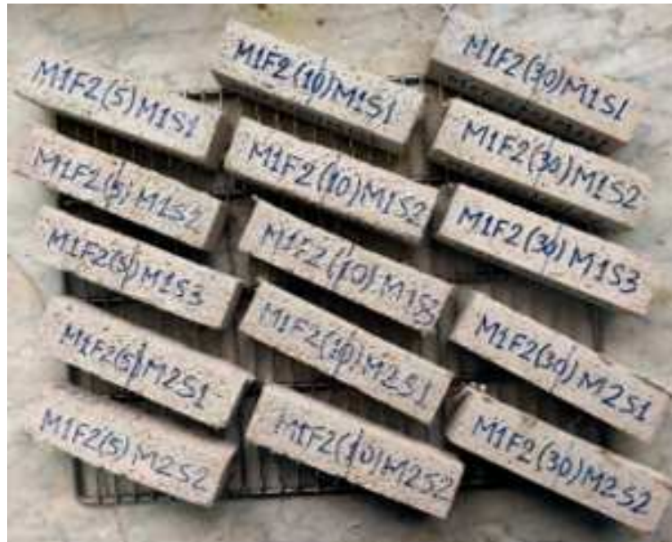
Fig. 5-10. Thermal mortar samples prepared using 2% fiber (with respect to the dry mortar mass), with 30 mm, 10 mm and 5 mm fiber lengths, respectively.
