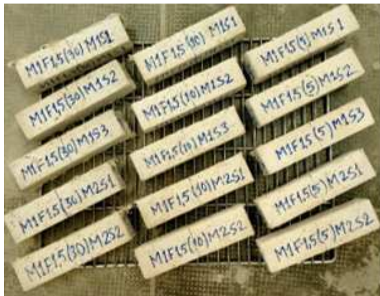
Fig. 5-9. Thermal mortar samples prepared using 1.5% fiber (with respect to the dry mortar mass), with 30 mm, 10 mm and 5 mm fiber lengths, respectively.
