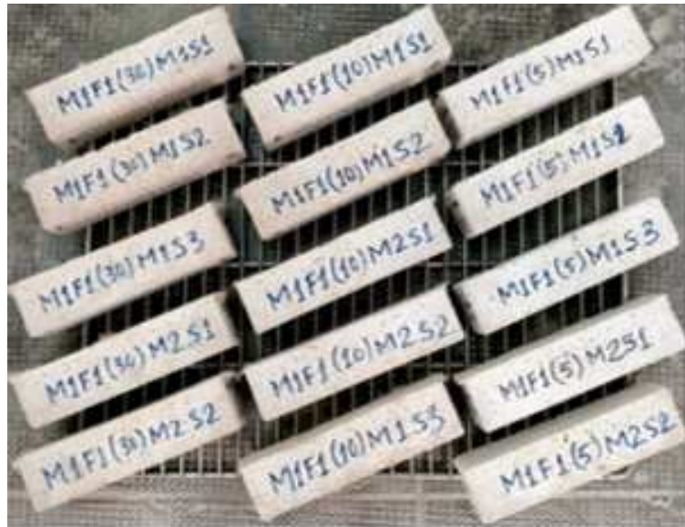
Fig. 5-8. Thermal mortar samples prepared using 1% fiber (with respect to the dry mortar mass), with 30 mm, 10 mm and 5 mm fiber lengths, respectively.
