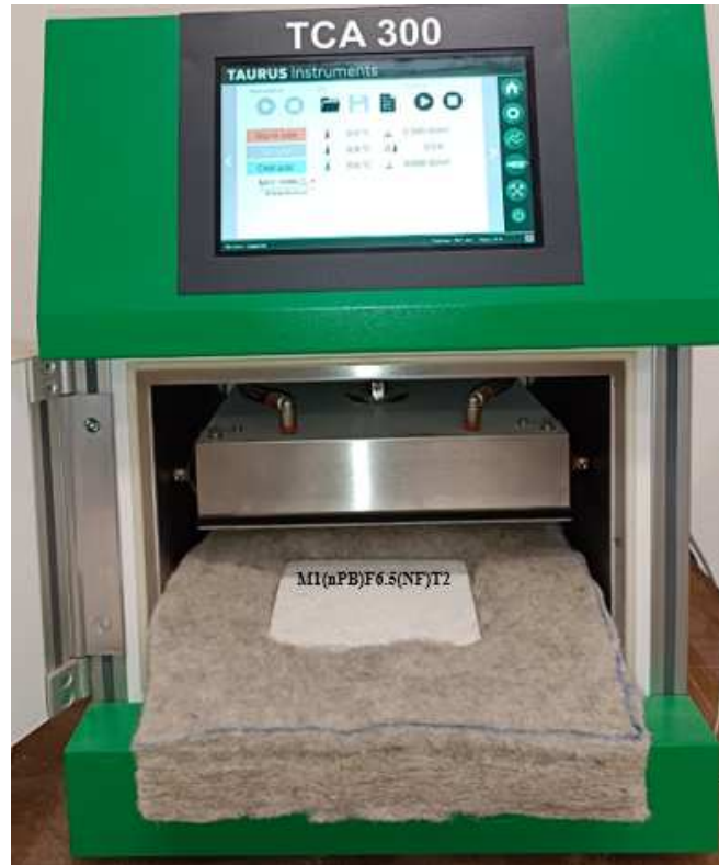
Fig. 8-8. Thermal conductivity test: sample M(nRA)F6.5(NF)T2 .
