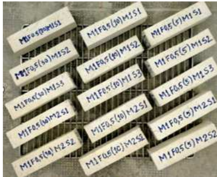
Fig. 5-7. Thermal mortar samples prepared using 0.5% fiber (with respect to the dry mortar mass), with 30 mm, 10 mm and 5 mm fiber lengths, respectively.
