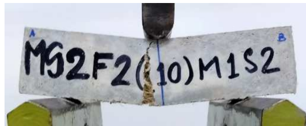
(c): MS2F2(10)M1S2 with 2% (with respect to mortar mass) and 10 mm fiber length.
