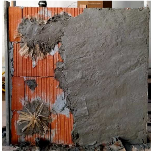
Fig. 7-16. HBW7 masonry wall upgraded with four jute diatoms and jute composite mortar (with 1% fiber (30 mm) with respect to dry mortar mass).
