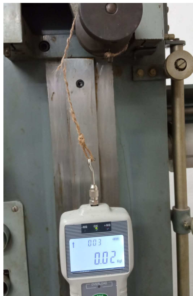
Fig. 4-26: Three yarns class 1 mm thread, after complete failure
