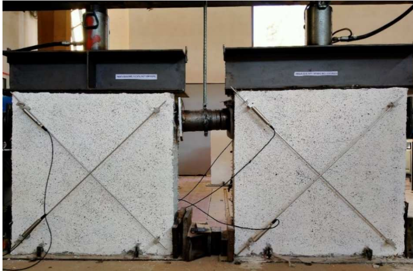
(a): Front view: masonry walls equipped with diagonal sensors.
