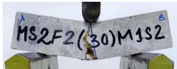
(b): MS2F2(30)M1S2 with 2% fiber (with respect to mortar mass) and 30mm fiber length
