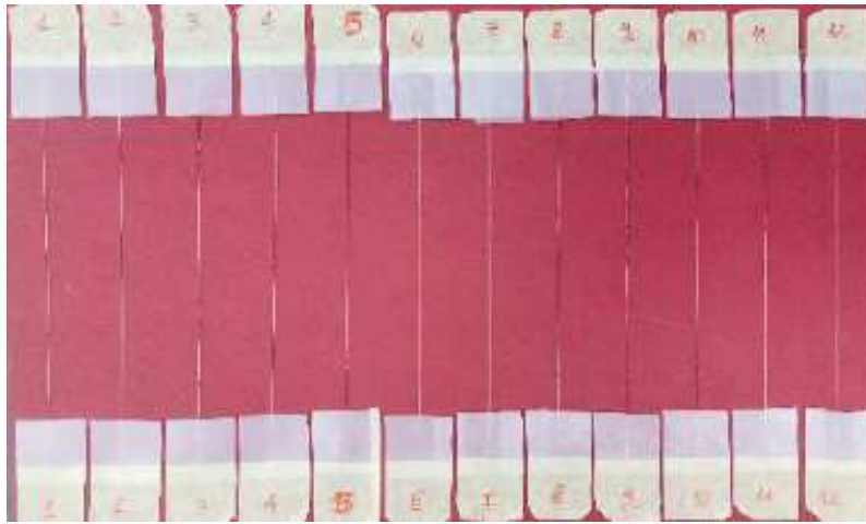
Fig.4-22. A total of 20 jute fibers used for tensile strength tests.
