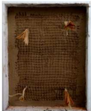
(c) TM application (lower layer) +Jute net placement
