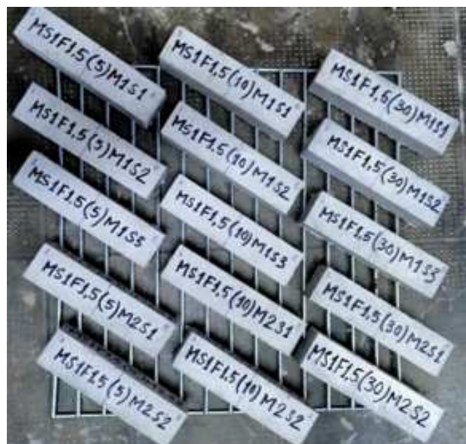
Fig. 5-13. Structural mortar samples prepared using 1.5% fiber (with respect to the dry mortar mass), with 30 mm, 10 mm and 5 mm fiber lengths, respectively.
