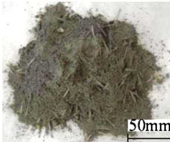
Fig. 2-10. Carbon fiber-mortar mix (Babaeidarabad et al 2014).
