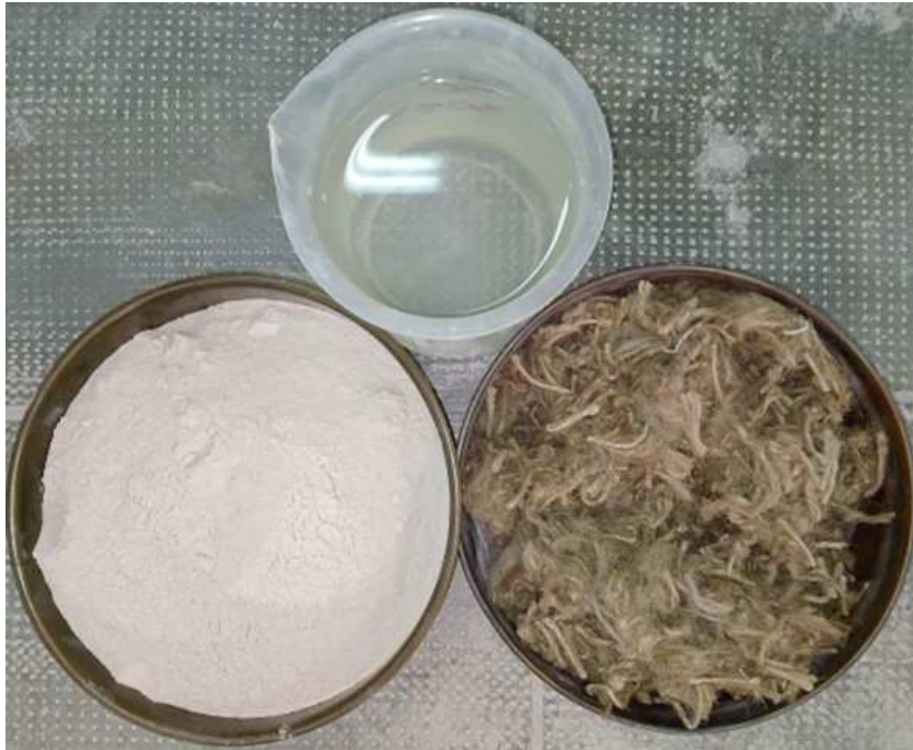
Fig. 8-2. Amount of water, thermal mortar (without PB) and recycled jute net fibers
