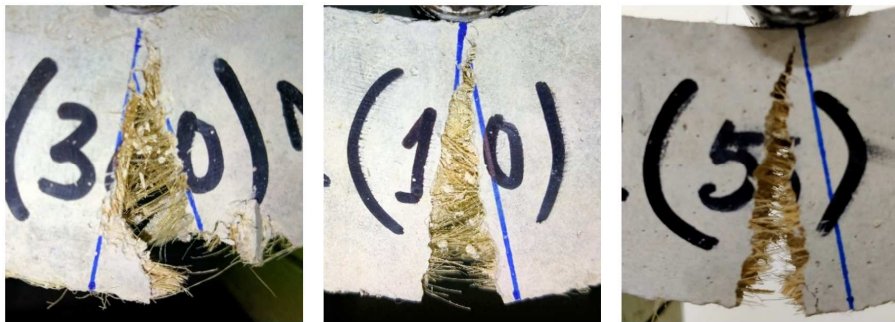
(a): 30mm fiber length (b): 10mm fiber length (c): 5mm fiber length
