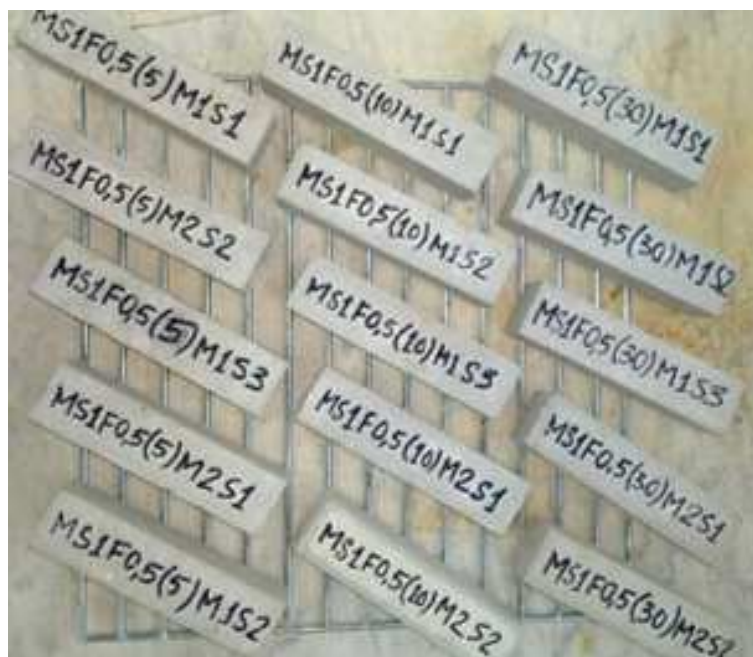
Fig. 5-11. Structural mortar samples prepared using 0.5% fiber (with respect to the dry mortar mass), with 30 mm, 10 mm and 5 mm fiber lengths, respectively.
