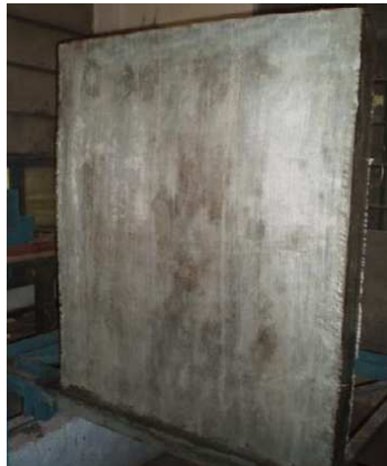
Fig. 2-46. GFRP wrapped wall (Sivaraja et al. 2013)
