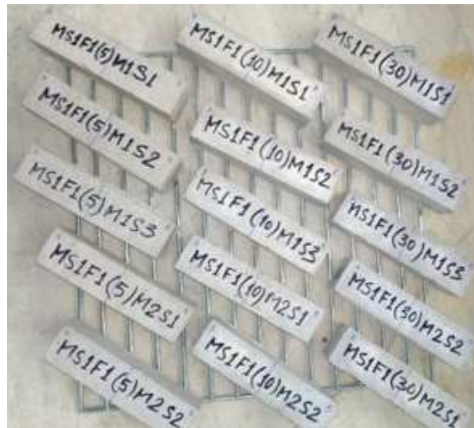
Fig. 5-12. Structural mortar samples prepared using 1% fiber (with respect to the dry mortar mass), with 30 mm, 10 mm and 5 mm fiber lengths, respectively.
