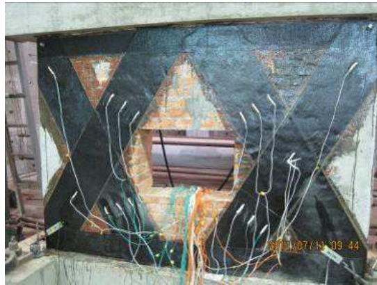
Fig. 2-51. BFRP-strengthened wall ( Lei et al. 2014 ).
