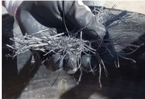
Fig. 2-12. Polypropylene fiber (Mustafaraj et al. 2020).
