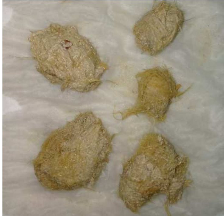
Fig.4-18. Fiber-balls formed as fibers come in contact with water.
