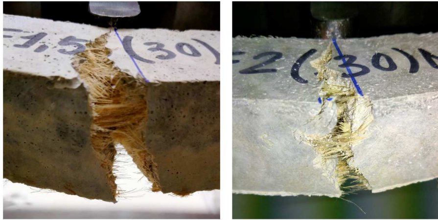
(a): Thermal composite mortar with 1.5% fiber (with respect to mortar mass) and 30mm fiber length (b): Structural composite mortar with 2% fiber (with respect to mortar mass) and 30mm fiber length
