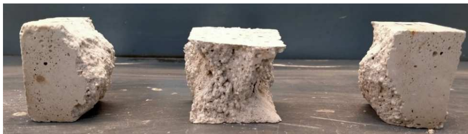
Fig. 5-41. A thermal mortar sample without fiber, after compression failure.
