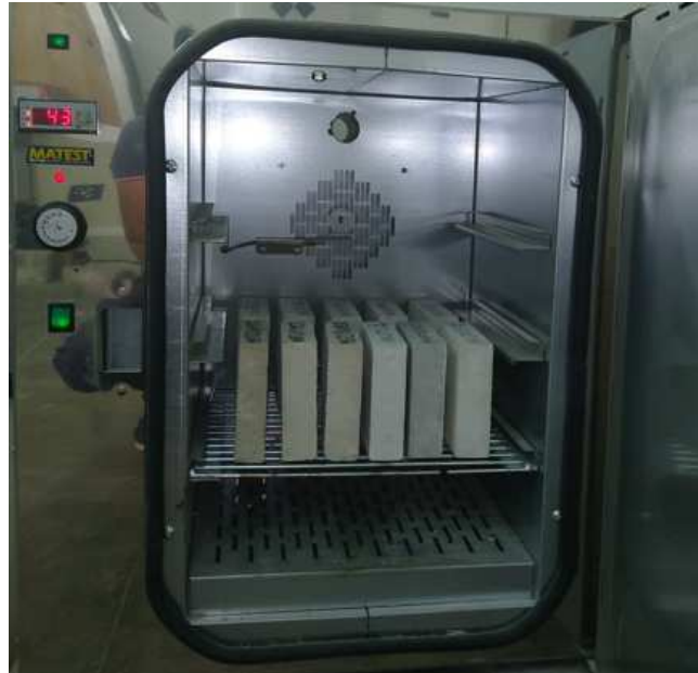
Fig. 5-22. Normal mortar (without fiber) and composite mortar samples are placed inside the oven for forced drying or moisture removal.
