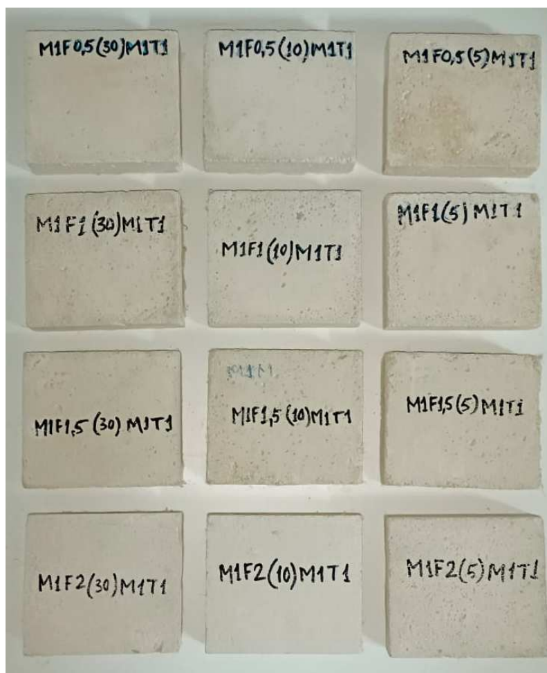
Fig. 5-19. Thermal composite mortar samples prepared using fiber percentages (0.5%, 1.0%, 1.5% and 2.0%) (with respect to the dry mortar mass) and fiber lengths (30 mm, 10 mm and 5 mm).
