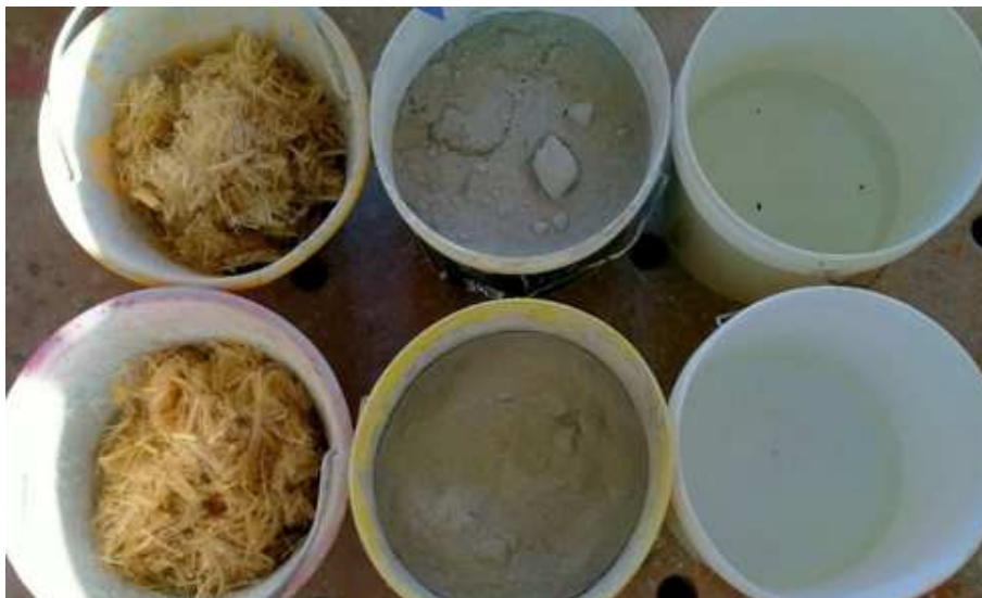
Fig. 7-4. Jute fiber of 30mm, structural mortar (SM), water for masonry wall upgrading.
