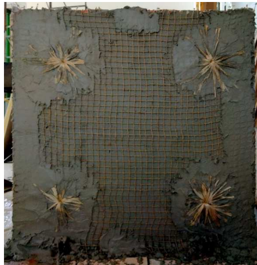
Fig. 7-15. HBW6 masonry wall upgraded with four jute diatons, 1x1 m 2 jute net (with mesh type 2.5cm x 2.5cm) and jute composite mortar (with 1% fiber (30mm) with respect to dry mortar mass).
