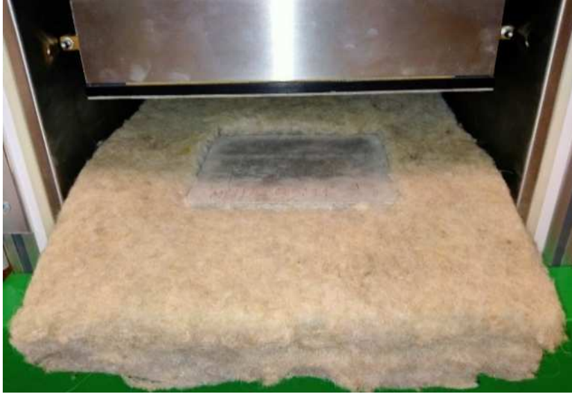
Fig. 5-27. Woolen heat guard is placed around the sample (MSIF0.5(30)TI)
