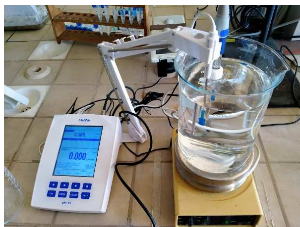
Fig.4-11. Case 3 - Preparation of alkaline solution with 9.5 pH
