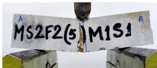
(d): MS2F2(5)M1S1 with 2% (with respect to mortar mass) and 5mm fiber length
