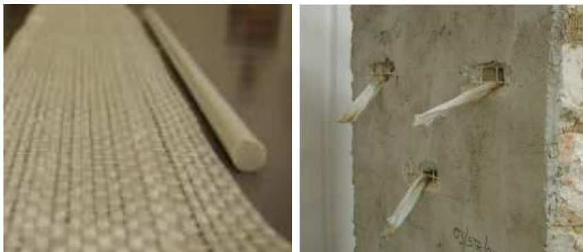
Fig. 2-21. GFRP bar and fiberglass sheet wrapped to use as horizontal connector (Mustafaraj et al. 2020).
