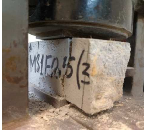
Fig. 5-42. Structural mortar: compression test failure for sample with 0.5% jute fiber (30mm) with respect to the dry mortar mass.
