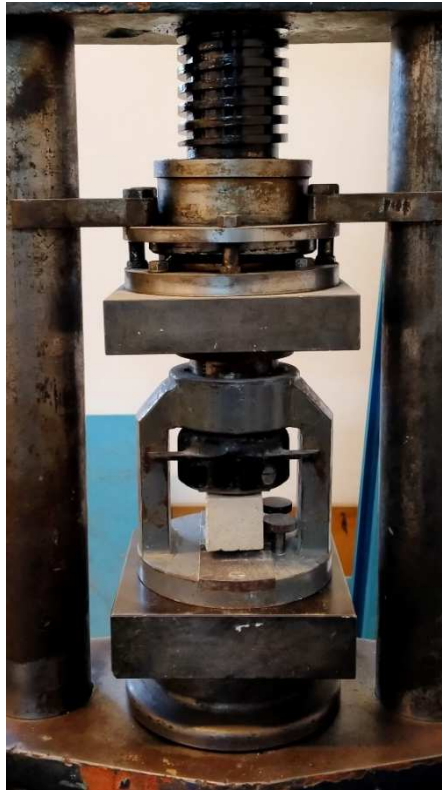
Fig. 5-17. Compression strength test (Sample MS1F1.5(30)M2S1).
