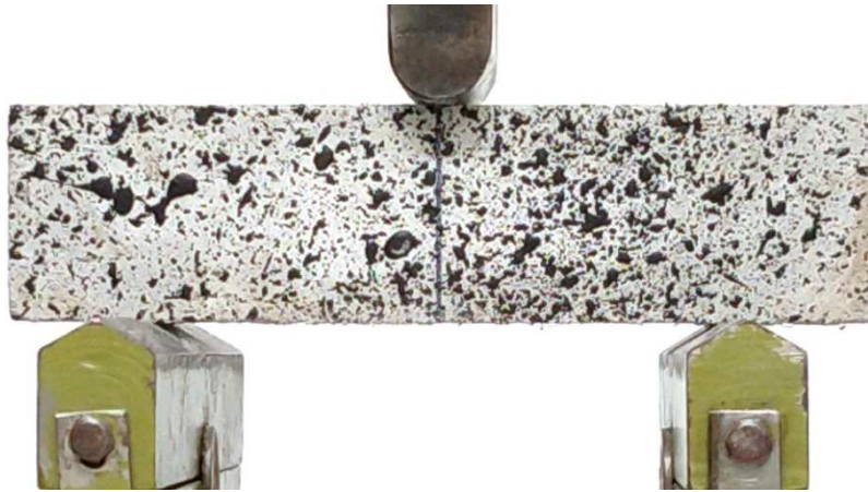
Fig. 9-3. Black spots/pattern surface of the sample MS1(SW)F0.5(5)MIS3.
