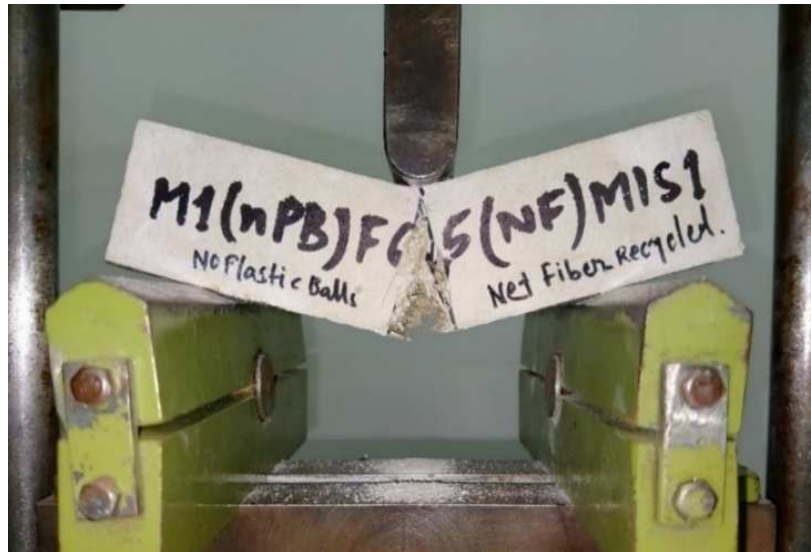
Fig. 8-5. Flexural strength test: sample M(nRA)F6.5(NF)MIS1.
