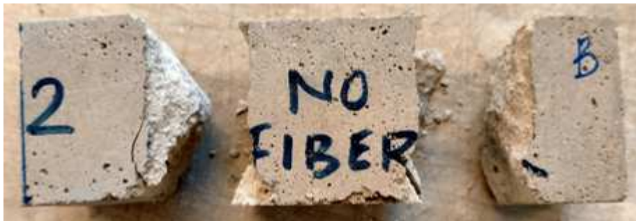
Fig. 5-40. A Structural mortar sample without fiber, after compression failure.
