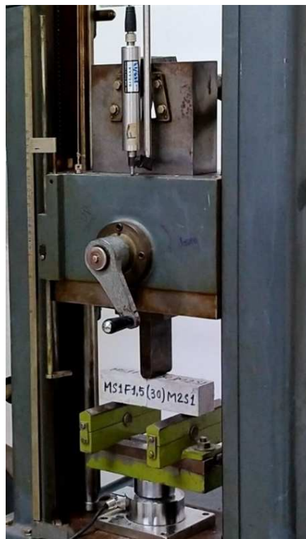
Fig. 5-15. Flexural strength test (Sample MS1F1.5(30)M2S1).
