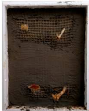
(c) SM application (lower layer) + Jute net placement
