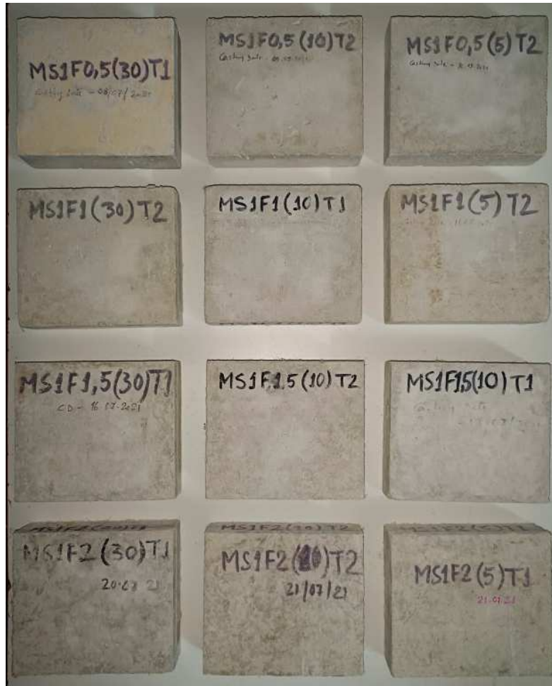
Fig. 5-20. Structural composite mortar samples prepared using fiber percentages (0.5%, 1.0%, 1.5% and 2.0%) (with respect to the dry mortar mass) and fiber lengths (30 mm, 10 mm and 5 mm).
