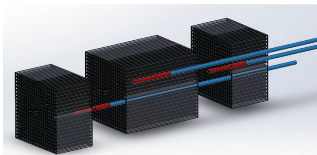
Figure 20: Isometric projection of the SiC monolith. INLET, MID, OUTLET acquisition position (AXIAL).
