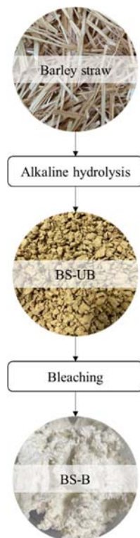
Figure IV.24 Schematic representation of pulping process on barley straw.
