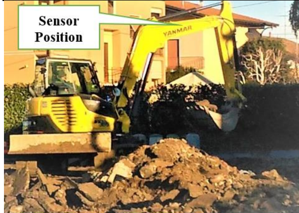
Figure V.17 Testing Inclinometer in Excavator
